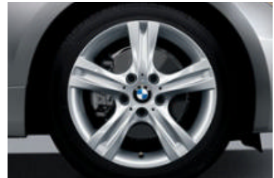
Star Spoke (Style 262) light alloy wheels and run-flat 2 performance tires. 3 In front: 17 x 7.0 wheels and 205/50 tires; in back: 17 x 7.5 wheels and 225/45 tires. 3 (included in 128i Sport Package)
