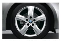
□ Star Spoke (Style 142) light alloy wheels with run-flat<sup>1</sup> all-season tires. In front:  $17 \times 7.0$  wheels and 205/50 tires; in back:  $17 \times 7.5$  wheels and 225/45 tires.<sup>3</sup>
