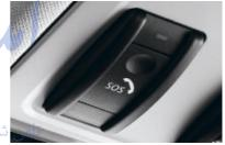
BMW Assist<sup>™</sup>1 and Bluetooth® system offers hands-free calling through your BMW-approved Bluetooth phone. The BMW Assist Safety Plan is included for four years, providing Automatic Collision Notification and more.
