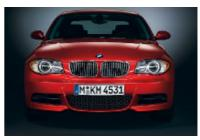
■ Front apron sits below the BMW double kidney-shaped grille with chrome slats. This feature, which brings a constant flow of fresh air to the engine, adds to the front's impressive athletic profile. The central air intake is flanked by two side air intakes that cool the brakes. Two side flaps accentuate the broad front.
