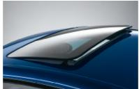
■ Two-way power glass moonroof with remote, expanded one-touch operation, slides backward or tilts up to let in as much fresh air and sky as you like, while a wind deflector helps keep the wind out. Includes a sliding interior sunshade.
