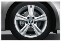
□ Star Spoke (Style 262) light alloy wheels and run-flat¹ performance tires.² In front: 17 x 7.0 wheels and 205/50 tires; in back: 17 x 7.5 wheels and 225/45 tires.³ (included in 128i Sport Package)
