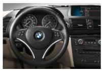
■ Three-spoke leather-wrapped multifunction steering wheel lets you keep both hands on the wheel while adjusting various comfort functions, such as controls for audio system, cruise control and hands-free phone controls.
