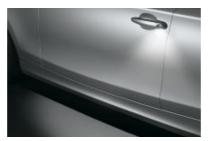
Ambiance light package includes lights in the exterior door handles that radiate downward whenever the doors are unlocked. They illuminate the area outside the doors for approximately 20 seconds to enable safe vehicle access in the dark. Also included are front and rear reading lights, front footwell illumination, vanity mirror lights for driver and front passenger, and ambiance interior lighting.
