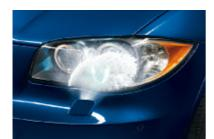
■ / □ High-intensity headlight washers help keep lights clean of ice, mud, road salt and other coatings, for maximum road lighting and enhanced driving safety. (Retractable washers std. on 135i; fixed washers included in 128i Cold Weather Package. 135i shown)
