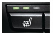
**Heated front seats** are a welcome feature for driver and front passenger in cooler weather. With the touch of a button, seat surface and backrest are heated and quickly radiate comfortable warmth in your choice of three settings. (Also available as a stand-alone option.)
