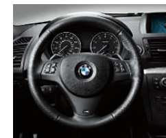
□ Three-spoke, leather-wrapped multi-function M sport steering wheel features a grip-enhancing wheel cover and distinctive M badging. Optional Voice command (included with optional Navigation system) can be used to change various selections and entries.
