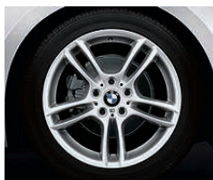
Double Spoke (Style 261M) light alloy wheels and run-flat 1 performance tires. 2 In front: 17 x 7.5 wheels and 215/40 tires; in back: 18 x 8.5 wheels and 245/35 tires.
