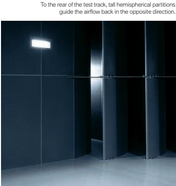
To the rear of the test track, tall hemispherical partitions guide the airflow back in the opposite direction.
