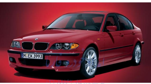
Thanks to modifications by driving enthusiast engineers at BMW, the 330i Performance Package brings track-inspired excitement to your daily drive. The suspension is even lower, stiffer and firmer than in the standard 330i. For greater adhesion, wheel camber is set at -0.5°, which results in a larger tire contact patch when cornering quickly. With a rear axle ratio that's 3.5% shorter, the car delivers noticeably crisper response and greater agility at all speeds.
