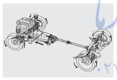
xDrive all-wheel-drive system monitors readings from the DSC sensors and the gas pedal to determine if over- or understeer is occurring. This data is then used to continually vary power distribution between the front and rear axles, ensuring agile, neutral and forgiving handling at all times. (standard in 328xi; not available in 328i or 335i)
