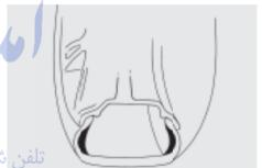
Run-flat tires allow speeds of up to 50 mph and travel from 30 to 150 miles after a loss of air pressure, dependent upon the passenger load and weight of articles being transported. In situations that would normally result in a flat, reinforced sidewalls help prevent the tires from collapsing or loosening from the rim. Please see your vehicle manual for additional details.
