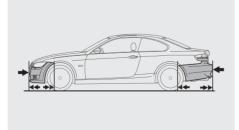
Impact-absorbing bumpers and compressible "crush tubes" front and rear help absorb the force of impact in collisions up to nine mph, helping to minimize damage to the vehicle's body and simplifying repairs. Only at higher impact speeds do structural supports begin to deform, dissipating impact energy to help protect occupants.
