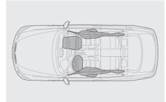
Six airbags, part of BMW's Advanced Crash Safety Management system, include "smart" dual-stage, dual-threshold front airbags that deploy at different forces, depending upon whether or not safety belts are worn; front-to-rear Head Protection System curtain-type airbags; and front-seat-mounted side-impact airbags.
