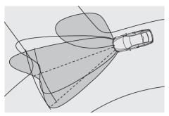
Xenon Adaptive Headlights illuminate the road ahead and to the side with brilliant clarity; Xenon headlights also have a dynamic autoleveling feature. BMW Adaptive Headlights illuminate the road around corners by directing the headlights into and through the bend, as soon as the vehicle begins cornering.
