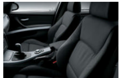
Eight-way adjustable front sport seats make the driving experience more enjoyable. Side bolsters can be power-adjusted to fit your back comfortably while helping to hold you firmly in place during cornering. (Eight-way power front sport seats with two-way manual headrests and thigh support: std. in 335i/335xi with Sport Package; opt. or included with Premium Package in 328i/328xi with Sport Package)
