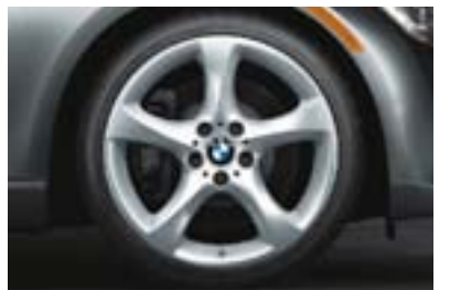
Star Spoke (Style 230) light alloy wheels with run-flat 1 performance tires. 2 In front: 19 x 8.0 wheels with 225/35 tires; in back: 19 x 9.0 wheels with 255/30 tires. (Optional on 335i, requires optional Sport Package.)
