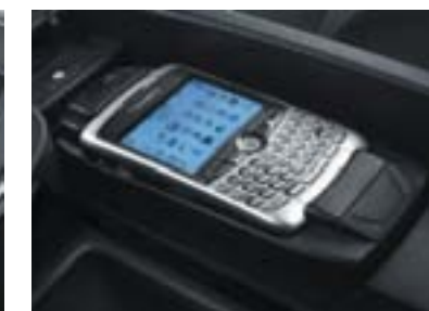
Snap-in adapter plays stored music, charges the phone and accesses the car antenna.
