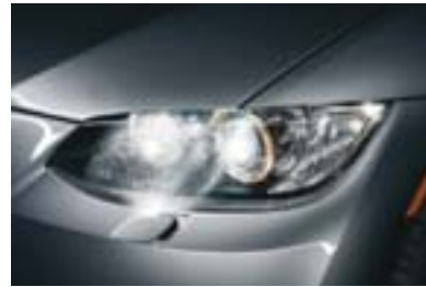
Retractable high-intensity headlight washers help keep lights clean of ice, mud, road salt and other coatings, for maximum road lighting and enhanced driving safety.
