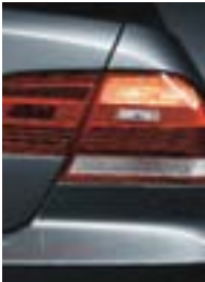
■ Adaptive Brake Lights increase vehicle visibility and signal the intensity of your braking action.
