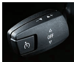
■ Dynamic Cruise Control lets you store and maintain a chosen speed above 20 mph. It is activated via the left-hand steering column switch, and deactivated by applying the brakes or via the switch. 2
