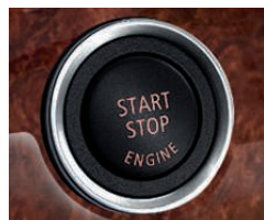
■ Engine Start/Stop button 1 and key fob control the engine. Upon inserting the key fob into the starter switch slot, and the electronic identification system confirms that it is the correct key fob, the engine can be started (or later, shut off) by pressing the Start/Stop button.
