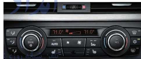
■ Automatic climate control system allows occupants to select a specific cabin temperature and choice of fan speeds, as well as automatic or manual airflow and recirculation. The automatic recirculation control activates whenever certain air pollutants are detected. The system also includes defrost/demist and MAX A/C functions.
