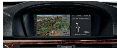
□ Navigation system features a high-resolution, glare-free monitor. Using GPS satellites in conjunction with data stored on an internal hard drive, a choice of detailed maps show – and tell – the directions to your desired destination. Enhancements include 3-D daytime and nighttime maps, zoom, travel planner and an Assistance Window. In many areas, it also provides Real Time Traffic Information on potential traffic problems along your route, and can even plan a detour around them. The Voice command feature can be used to change radio stations and audio selection, Navigation system destinations, and (accessory) telephone entries.
