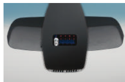
■ Rain sensor measures the amount of rain. In "intermittent" windshield wiper mode, it automatically adjusts the wiping interval as needed. Includes Automatic headlight control (not shown), which activates headlights by means of a sensor that responds to darkness. The rain sensor is also integrated into the braking system as part of the Brake Drying feature.
