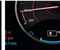
Auto Start-Stop function – and on the BMW ActiveHybrid 3, the Hybrid Start-Stop function – switches off the engine automatically during brief stops, such as at red lights, to reduce fuel consumption. A symbol displayed in the rev counter indicates that the function is active.
