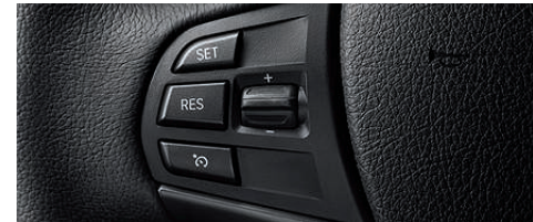
Dynamic Cruise Control 3 lets you set and keep to a chosen speed above 20 mph, including automatic application of the brakes when driving downhill. It is activated and regulated via controls positioned on the left side of the steering wheel, and deactivated by applying the brakes or switching off the feature.
