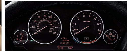
Instrument panel features a red backlit speedometer and tachometer. Centered between the two easy-to-read analog instruments is the on-board computer with liquid crystal display providing additional important driving information.
