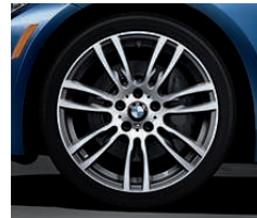
Star Spoke (Style 403M) light alloy wheels and run-flat 1 performance tires. 2 In front: 19 x 8.0 wheels and 225/40 tires; in back: 19 x 8.5 wheels and 255/35 tires.
