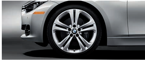
Double Spoke (Style 401) light alloy wheels and run-flat 1 performance tires. 2 In front: 19 x 8.0 wheels and 225/40 tires; in back: 19 x 8.5 wheels and 255/35 tires.
