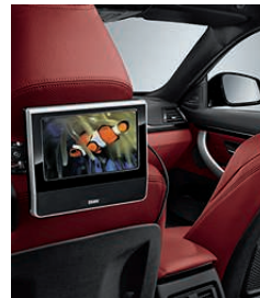
BMW Tablet DVD System. Portable screens (with integrated DVD player) play DVDs, CDs, and include an integrated USB interface and card slots.
