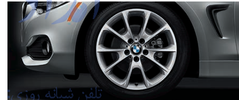
V Spoke (Style 398) 4 18 x 8.0 front, 18 x 8.5 rear light alloy wheels and 225/45 front, 255/40 rear run-flat 1 performance tires . 2,3 (Requires M Sport brakes; includes increased top-speed limiter.)
