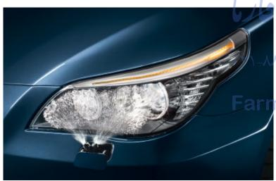
Retractable **high-intensity headlight washers** help keep lights clear of ice, mud, road salt and other coatings, for maximum road lighting and enhanced driving safety.
