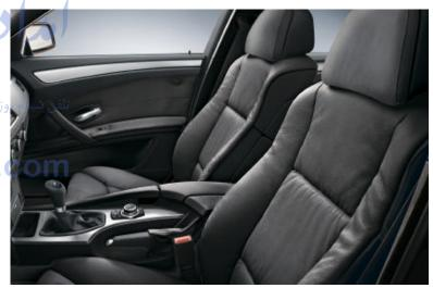
20-way power multi-contour front seats provide optimum lateral support during tight cornering, while remaining exceptionally comfortable when driving over long distances. In addition to Active Head Restraints, the seats offer individual power adjustment for backrest and seat-bottom angle; forward/backward and up/down position; thigh, upper back and lumber support; and adjustable sides.
