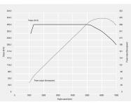
Portrait of a masterpiece: the 3.0-liter twin-turbo engine produces 300 horsepower at 5800 rpm, and quickly develops 300 lb-ft of torque at 1400 rpm, which continues without fading through to the 5000 rpm range. With such a broad range of powerful torque, you can enjoy smooth, robust acceleration in any qear, at any speed.
