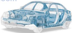
Under the surface of the 5 Series Sedan is a comprehensive array of passive safety features. The extremely rigid body routes impact forces around the passenger cell. In the event of a side impact, the interlocking door anchoring system offers added protection. Not shown: A full complement of airbags – four in front, optional side-impact airbags at the rear – includes Head Protection System, which helps cushion and protect the heads of occupants seated by the doors.
