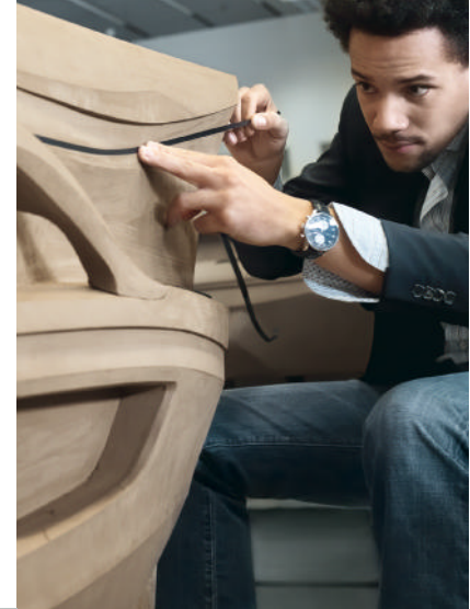
Interior designer Oliver Heilmer checking the lines and dimensions of the body on the clay model.
