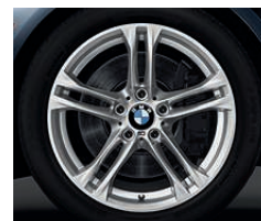
Double Spoke (Style 613M) light alloy wheels. With run-flat¹ performance tires²: 18 x 8.0 front, 18 x 9.0 rear and 245/45 front, 275/40 rear tires. (Includes increased top-speed limiter.) With run-flat¹ all-season tires³: 18 x 8.0 and 245/45 tires.
