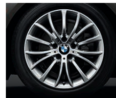
Multi Spoke (Style 454) 18 x 8.0 light alloy wheels and 245/45 run-flat¹ all-season tires.²
