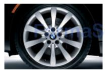
☐ 19 x 8.5 Star Spoke (Style 218) cast alloy wheels and 245/40R-19 run-flat performance tires.<sup>1</sup>
