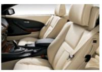
■ Eight-way power front seats with four-way power lumbar support and two-way adjustable headrests firmly support the driver and front passenger over long distances. Front-seat bolsters help eliminate "submarining" during sudden stops. Includes Active Head Restraints and driver's-seat memory function for settings. (shown in Cream Beige Dakota Leather upholstery)
