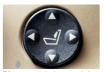
■ Four-way power lumbar support for front seats offers comfort and lower back muscle support. Lumbar support can be adjusted four ways: up/down and in/out.
