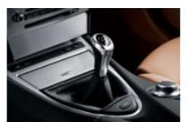
■ 6-speed manual transmission delivers a precise, athletic feel that's responsive to your personal driving style. This is due, in part, to the enhanced synchronization of shifts from neutral to each gear. The gearbox adds to the sporty feel, with a shortened shift lever and throw.
