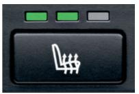
☐ **Heated front seats** are a welcome feature for driver and front passenger in cooler weather. With the touch of a button, seat surface and backrest are heated and quickly radiate comfortable warmth in your choice of three settings. (Opt. and included in Cold Weather Package)
