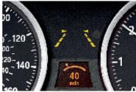
□ Lane Departure Warning feature<sup>2</sup> alerts the driver by discreetly vibrating the steering wheel if the vehicle crosses lane markings without using the directional signal.
