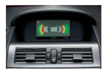
■ Park Distance Control (PDC), front and rear, helps parking and maneuvering in tight spaces. The distance between your vehicle and an obstacle is indicated by an acoustic signal that increases in intensity as your bumper approaches the object, turning into a constant tone when the distance closes to 12 inches. A visual representation is also projected on the iDrive Control display.
