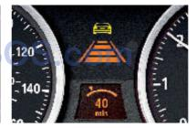
□ Active Cruise Control (ACC) with Stop & Go allows the driver to preset a desired speed. When ACC recognizes slower-moving vehicles ahead, it automatically brakes to maintain a preset distance, then resumes the set speed as soon as possible.¹ In traffic, Stop & Go can reduce the speed down to a standstill. (requires optional Sport Automatic transmission)
