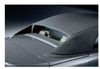
■ Automatic fin roof Convertible softtop is triple-lined and fully automatic. Simply press a button at the front of the center console to raise or lower. The top automatically unlatches from the header and folds down neatly. An interior lining helps reduce wind noise and enhances insulation. The heated glass rear window can be raised or lowered independently of the softtop. Available in Black or Gray. (650i Convertible only)
