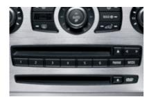
■ Six programmable memory keys offer convenient storage of your most frequently accessed iDrive settings, such as favorite radio stations, Navigation system addresses, phone numbers and more.
