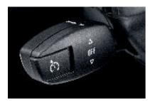
■ Cruise control lets you store and maintain a chosen speed above approximately 18.5 mph (activated via the left-hand side steering column switch). Cruise control is deactivated by applying the brakes or moving the lever.
