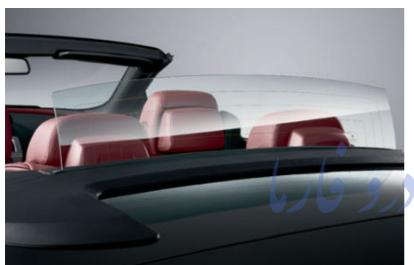
■ Heated glass rear window in the 6 Series Convertible can be raised independently of the softtop to reduce air turbulence and create a quieter cabin when driving at higher speeds. When driving in slower traffic, or when the softtop is raised, the window can also be lowered out of sight. (650i Convertible only)
