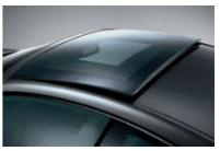
■ Tilting glass panel roof gives the interior an even brighter, more spacious feel. For greater ventilation, it tilts up; an electric sliding interior roofliner keeps the hot sun out. (650i Coupe only)
