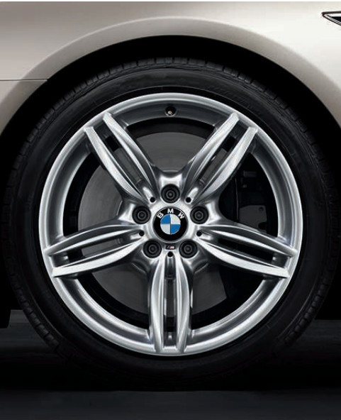
Double Spoke (Style 351M) 19 x 8.5 front, 19 x 9.0 rear light alloy wheels with 245/40 front and 275/35 rear run-flat 1 performance tires 2
