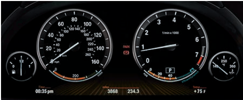
Instrument cluster displays speedometer, tachometer, fuel gauge and engine oil temperature. Below the four dials is a high-resolution Info Display that shows data such as current fuel consumption, range, on-board computer functions, mileage and trip information. Black Panel Display technology shows the instrument cluster as a matte black surface when the ignition is switched off, with only the chrome rings of the circular instruments visible in 3-D. When the ignition is switched on, the chrome rings turn into full circles, and the dials and displays appear. Turning on the ignition also activates the Check Control messages.
