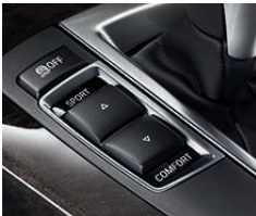
Driving Dynamics Control adjusts driving characteristics by pressing a button to select one of four settings. Choosing COMFORT, NORMAL, SPORT or SPORT+ mode adjusts the engine-throttle response, shift characteristics and power-steering assist. Another button disengages the traction control feature when driving on sand, gravel, or deep or packed snow.
