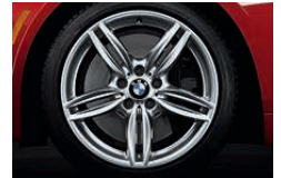
Double Spoke (Style 351M) 19 x 8.5 front, 19 x 9.0 rear light alloy wheels with 245/40 front and 275/35 rear run-flat performance tires . 1
