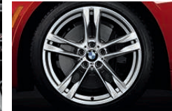
Double Spoke (Style 373M) 20 x 8.5 front, 20 x 9.0 rear light alloy wheels with 245/35 front and 275/30 rear run-flat performance tires . 1
