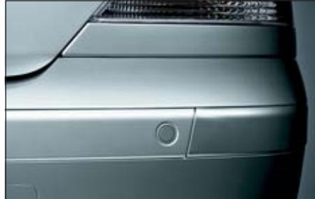
■ **Park Distance Control** uses ultrasonic sensors in both bumpers to help you judge the distance to cars and unseen objects when parking. The beeping becomes faster as your bumper approaches the object, turning into a constant tone when it's less than 12" away.
