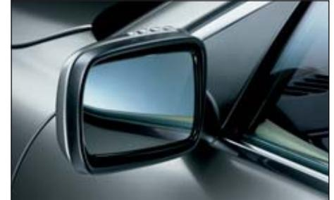
■ **Auto-dimming, power side-view mirrors** are tinted blue, with body-color mirror housing. The mirrors automatically heat up when the defroster is turned on.
