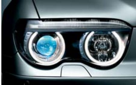
■ **Xenon low- and high-beam headlights** illuminate the road ahead and to the side with brilliant clarity. These headlights also have an auto-leveling feature. **BMW Adaptive Headlights** provide road illumination around corners by directing the headlights into and through the bend as soon as the vehicle begins cornering.
