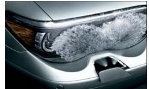
■ **Retractable high-intensity headlight washers** help keep lights clean of ice, mud, road salt and other coatings, for maximum road lighting and enhanced driving safety.
