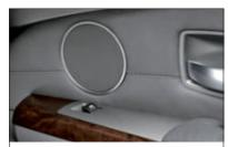
■ Standard audio system generates powerful sound through 10 speakers, including midrange speakers in each front door and each side of rear hat-shelf; tweeters in the front door mirror triangles; and subwoofers under the front seats. (750i/750Li)
