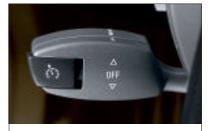
■ Programmable cruise control can be pre-programmed with up to six cruising speeds. It can retrieve them at any time by pushing the stalk forward or pulling it back. Pre-programmed speeds appear as arrows along the speedometer scale.
