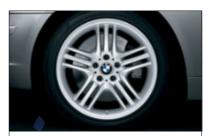
■ 19" Star Spoke (Style 89) cast alloy wheels and performance tires.¹ Front: 19 x 9.0 wheels, 245/45R-19 tires; rear: 19 x 10.0 wheels, 275/40R-19 tires. (std. on 760Li; not available on 750i/750Li)
