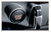
■ Engine Start/Stop button and remote key control the engine. First insert the remote key into the starter switch slot. After the electronic identification system confirms that it is the correct remote key, you can start or turn off the engine by pressing the Start/Stop button.
