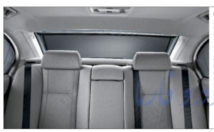
■/□ Power sunshades for the rear window and rear side windows provide optimum protection from sun glare and heat, while allowing extra privacy for rear-seat occupants. Rear shade raises or lowers at a touch; if the switch is held down, the side shades (two shades per each rear side window) join in the motion. Each rear door has switches that control all the shades. A child-safety switch disables operation. (std. in 760Li; opt. in 750i/750Li and included in 750i/750Li Luxury Seating Package)
