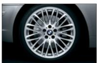
□ 20" Double Spoke (Style 149) cast alloy wheels and performance tires.¹ Front: 20 x 9.0 wheels, 245/40R-20 tires; rear: 20 x 10.0 wheels, 275/35R-20 tires. (included in 750i/750Li Sport Package)
