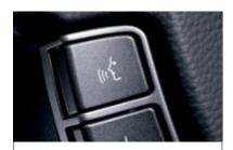
■ Voice Activation allows you to activate numerous Navigation system functions, record up to five minutes of notes, and dial hands-free. The Voice Activation button must be pressed before each use, so conversations won't accidentally activate the phone or other systems.
