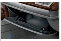
■ Glove compartment is thoughtfully illuminated and includes a convenient removable, rechargeable flashlight.
