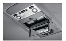
■ Vanity mirror is positioned in the rear roof lining for the convenience of back-seat occupants. Centrally positioned, it swivels and illuminates.
