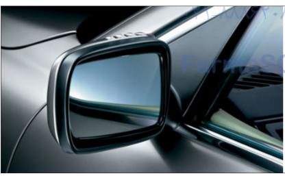
■ Exterior side-view mirrors are power adjustable, heated, and automatically dim when reflecting bright lights – helping to eliminate glare when driving at night. Both body-color mirrors have a folding function, moving in and folding out again at the touch of a button.
