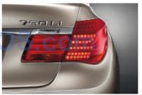
■ Adaptive Brake Lights, shown in the redesigned taillight cluster, consist of layered red LED indicators that offer quicker, heightened vehicle visibility by signaling the intensity of your braking action, thereby warning following drivers to brake quickly.
