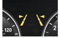
□ Lane Departure Warning system, included in the optional Driver Assistance Package, uses a camera to identify when the vehicle is getting close to a road marking, and warns the driver immediately by sending a mild vibration through the steering wheel. The system can be switched on and off via a button to the left of the steering wheel.
