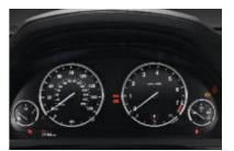
■ Dashboard with four analog instruments shows speed, rpm, fuel level and engine oil temperature above a high-resolution, wideformat Info Display. Also shown, as a graphic display, are the current fuel economy and range, as well as trip computer functions, an odometer and a daily trip recorder.
