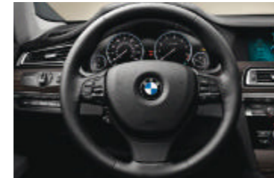
Three-spoke leather-wrapped multi-function M sport steering wheel features a slightly smaller diameter, thick padding, and special thumb rests for a comfortable grip during sporty driving maneuvers.
