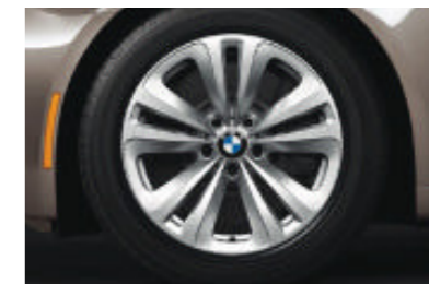
■ Double Spoke Star (Style 234) 18x8.0 light alloy wheels with 245/50 run-flat 1 all-season tires.
