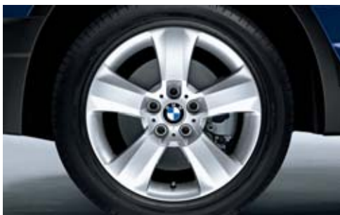
The X3 3.0i Sport Package includes Star Spoke (Styling 113) 18 x 8.0 alloy wheels and 235/50 R-18 all-season tires. (Spare is a space-saver wheel and tire)
