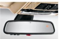
The automatic-dimming inside rear-view mirror darkens in response to the bright headlights of vehicles behind you. An easy-to-read digital compass, integrated into the mirror, is a convenient way to constantly keep your bearings while driving. A three-button Universal garage-door opener can be programmed to open garage doors and activate various remote convenience functions.
