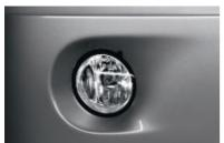
■ Halogen free-form foglights are cleanly integrated into the front air dam, illuminating the road ahead in bad weather and poor visibility. They also provide another practical feature, Cornering Lighting. When the system senses you are making a turn – based on your steering angle and speed – a reflector mechanism in the foglight housing casts additional lighting up to 90 degrees in the direction of the turn. This enhances visibility and recognition of people and objects.
