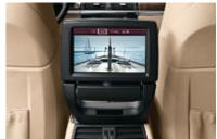
□ Rear-seat entertainment system lets passengers in the rear cabin watch DVDs or listen to their choice of CDs through headphone jacks. The system features a fold-down 8-inch color screen and headphone jacks; it can be controlled via a wireless remote control or manually by the rear-seat passengers.
