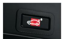
Automatic tailgate can be opened using the remote. When closed, via a button in the tailgate handle, the cargo area cover also automatically lowers. Maximum opening height can be programmed through iDrive. (Caution: measure height of garage ceiling before setting maximum opening height.)
