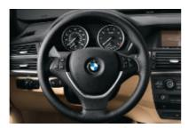
Three-spoke leather-wrapped multifunction sport steering wheel, featuring power tilt/telescoping adjustments, lets you keep both hands on the wheel while adjusting controls for cruise, audio and Bluetooth® enabled mobile phones.<sup>2</sup>
