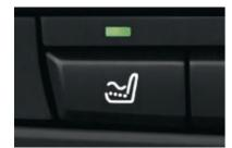
Active driver's seat helps decrease stiffness or fatigue on long trips. When activated, the driver's seat surface is continuously and imperceptibly raised and lowered from side to side, keeping your spine in motion and exercising various support muscles.
