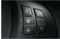
**Heated steering wheel** is a feature that, like heated seats, becomes a "must-have" once it's experienced. The heating switch is conveniently located on the multi-function steering wheel.
