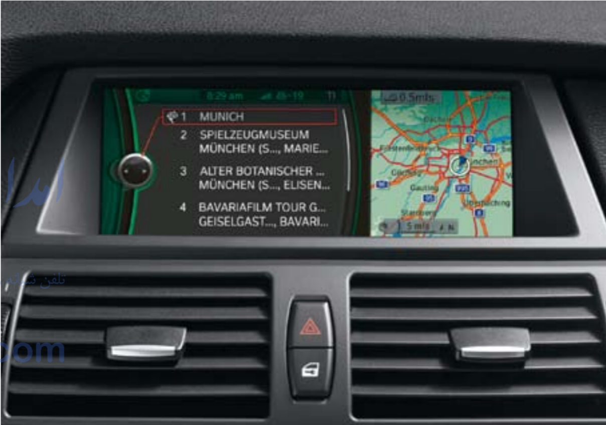
□ Navigation system 8.8" monitor uses transreflective technology to greatly reduce sun glare. As a result, you enjoy vivid colors and easy-to-read type, whether in bright daylight or poor light conditions. The monitor is ergonomically positioned for minimum visual distraction while driving. In many large cities, the Navigation system can display and describe the Real Time Traffic Information around your BMW. If congestion is on your planned route, the system can often plan a detour around it. (Optional Navigation system is also included in Technology Package.)
