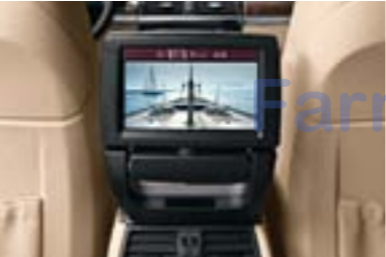
□ Rear-seat entertainment system lets passengers in the rear cabin watch DVDs or listen to their choice of CDs through headphone jacks. The system features a fold-down 8-inch color screen and headphone jacks; it can be controlled via a wireless remote control or manually by the rear-seat passengers.
