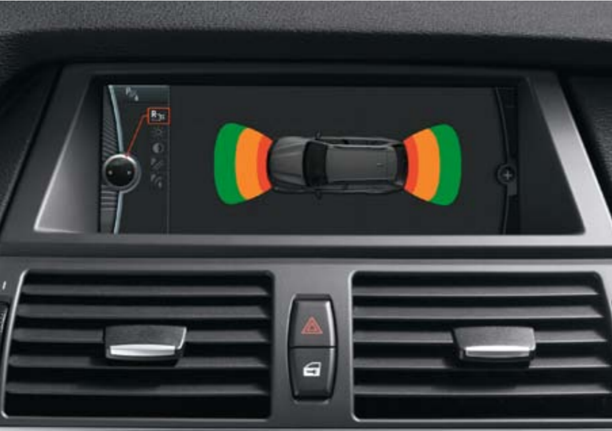
□ Park Distance Control uses eight sensors – four in the front, four in the rear – to help you judge how close you are to other cars and unseen objects when parking. The warning beeps come faster as the bumper approaches the object, turning into a constant tone when the distance is less than 12 inches.
