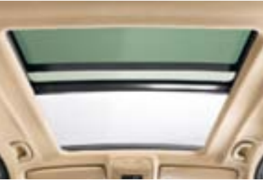
■ Extra-large dual-glass-panel Panoramic moonroof lets the sun and stars shine in, whether it is open or closed. Easy-use features include a power slide and lift control, a comfort opening/closing function, a wind deflector to help keep the wind out, and a power sunshade to shield passengers from excessive glare and heat.
