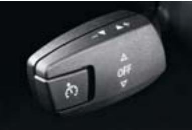
■ Dynamic Cruise Control lets you store and keep to a chosen speed above 20 mph, and automatically applies the brakes downhill. It is activated via the left-hand steering column switch, and deactivated by applying the brakes or via the switch. 3
