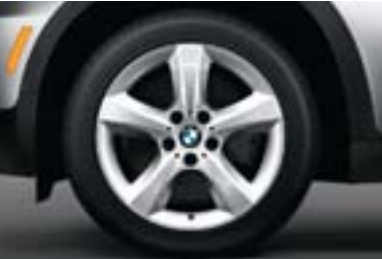
■ Star Spoke (Style 210) 18 x 8.5 light alloy wheels and 255/55 run-flat 1 all-season tires are standard on the X5 xDrive30i and X5 xDrive35d.
