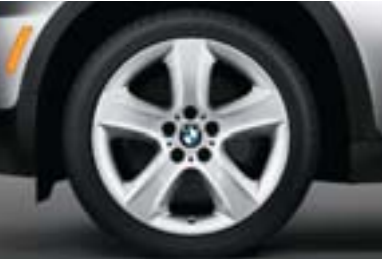
□ Star Spoke (Style 212) 19 x 9.0 light alloy wheels and 255/50 run-flat 1 all-season tires are included in the X5 xDrive30i and X5 xDrive35d Sport Activity Package.
