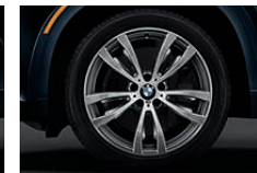
Double Spoke (Style 469M) 20 x 10.0 front, 20 x 11.0 rear light alloy wheels and 275/40 front, 315/35 rear run-flat 1 performance tires. 2,3 (Includes increased top-speed limiter.)
