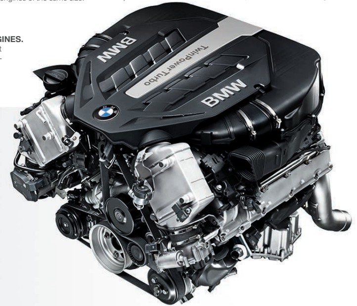
445-hp BMW TwinPower Turbo V-8 engine.
