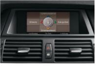
■ Glare-free Control display screen, linked with the iDrive and Navigation system, renders clear images and text. The surface of this new-generation display is equipped with transreflective technology, ensuring legibility by automatically making adjustments to the brightness or background lighting in brightor poor-light conditions.
