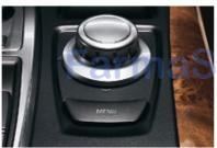
■ iDrive Controller, conveniently located on the center console, allows access to a variety of functions that are displayed on the Control display screen. The turn/press button enables front-seat occupants to access the menu system and fine-tune settings for climate control, the audio system, Navigation system<sup>4</sup> and communication through BMW Assist.™1
