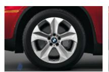
■ 19 x 9.0 Star Spoke (Style 232) light alloy wheels and 255/50 run-flat all-season tires are standard on the X6 xDrive35i. (Run-flat tires do not come equipped with a spare tire and wheel.)
