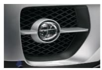
■ Halogen free-form foglights are cleanly integrated into the front air dam, illuminating the road ahead in bad weather and poor visibility. They also provide another practical feature: Cornering Lights. When the system senses you are making a turn – based on your steering angle and speed – a reflector mechanism in the foglight housing casts additional lighting up to 90 degrees in the direction of the turn. This enhances visibility and recognition of people and objects.
