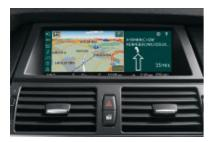
■ / □ Navigation system covers the U.S. with a single DVD. The glare-free monitor is mounted neatly into the dashboard for easy viewing. Using GPS satellites and DVD technology, a map of your area appears on the dash monitor, showing – and telling – the directions to your desired destination. It also provides Real Time Traffic Information (where available) on potential traffic problems and solutions. (standard in X6 xDrive50i; optional and included in X6 xDrive35i Technology Package)
