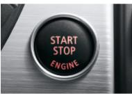
■ Engine Start/Stop button<sup>3</sup> and remote key control the engine. First, insert the remote key into the starter switch slot. After the electronic identification system confirms that it is the correct remote key, you can start (or later, turn off) the engine by pressing the Start/Stop button.
