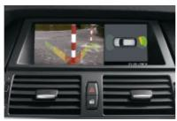
□ Rear-view camera is activated automatically by shifting into reverse gear, or manually by pressing the parking-assist button. The color display shows a real camera image that may include "static" and "track" lines to help you when backing up or parallel parking. (optional; included in the X6 xDrive35i Technology Package)
