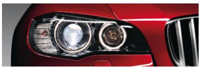
■ Xenon Adaptive Headlights optimize road illumination when the X6 enters a turn or corner, helping to enhance visibility when driving at night. Sensors continuously monitor the angle of the steering wheel to determine the direction in which the X6 is heading. The outer headlights swivel accordingly, up to 15 degrees left or right.
