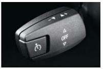
■ Dynamic Cruise Control lets you store and keep to a chosen speed above 20 mph, and automatically applies the brakes downhill. It is activated via the left-hand steering column switch, and deactivated by applying the brakes or via the switch.<sup>5</sup>
