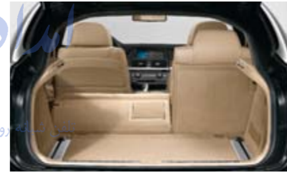
When equipped with the Premium Package, two lashing rails with four sliding lashing eyes, as well as additional lighting, make it easy to see and secure cargo safely and quickly.
