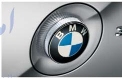
■ Side indicator lights with white lenses. When flashing, the light radiates outward from behind BMW's signature roundel.
