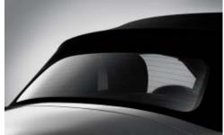
■ Heated, glass rear window and easy, onehand release/lock operation allow the softtop to make the Z4 Roadster into a comfortable allweather car. Thanks to a new folding sequence, the softtop's front section doubles as a tonneau cover and lies flush for a neat appearance. When the top is up, its variable storage compartment can be used to stow added cargo.
