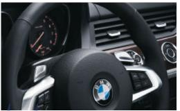
☐ Steering wheel-mounted paddle shifters, included with the 6-speed Sport Automatic and 7-speed Double Clutch Transmission, allow you to shift gears manually without using a clutch.
