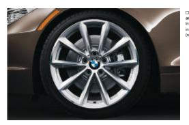
U Spoke (Style 296) light alloy wheels and run-flat performance tires.1 In front: 19 x 8.0 wheels and 225/35 tires; in back: 19 x 9.0 wheels and 255/30 tires. (opt. in Z4 sDrive35i with Sport Package)
