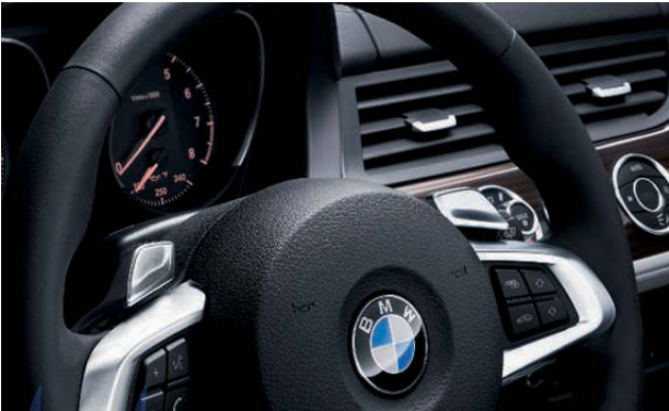
■/□ Steering wheel-mounted paddle shifters allow you to shift gears manually without using a clutch, and are included with the 7-speed Double Clutch Transmission and 6-speed Sport Automatic. □ Heated steering wheel makes gloves unnecessary in cold-weather driving. A flick of the switch quickly warms the steering wheel to the perfect temperature.
