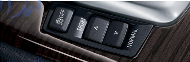
■ Driving Dynamics Control allows you to tailor the Z4's performance by selecting NORMAL, SPORT or SPORT+ driving modes at the touch of a switch. This changes throttle response, steering assist, suspension damping (with optional Adaptive M Suspension) and automatic transmission shifting (if so equipped). Additionally, you can deactivate Dynamic Stability Control (DSC) or switch to Dynamic Traction Control (DTC), which allows wheelslip within defined limits when driving in deep snow, or for a sportier driving style. ■/□ Adaptive M Suspension lowers the chassis by 0.4 inches and electronically adjusts the dampers from sportingly tight to relaxed and comfortable, for greater agility and precise response.
