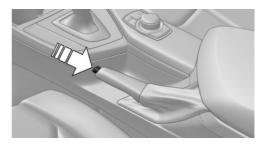
Raise lever slightly, press the button and guide the lever down.
