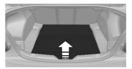
The tow fitting is located in the onboard vehicle tool kit under the cargo floor panel.
