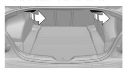
2. The unlocked backrest moves forward slightly.
