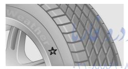
For each tire size, the manufacturer of your vehicle recommends certain tire brands. These can be identified by a star on the tire sidewall. With proper use, these tires meet the highest standards for safety and handling.
