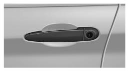
Unlock or lock the driver's door via the door lock using the integrated key, refer to page 34. The other doors must be unlocked or locked from the inside.
