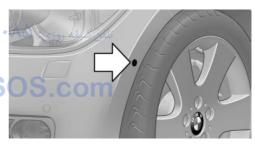
The four ultrasound sensors for measuring parking spaces are located in the front and rear on the side of the vehicle.
