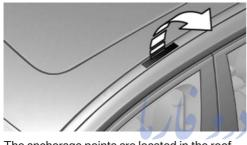
The anchorage points are located in the roof drip rail above the doors.
