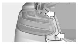
Grasp the handle with one hand, arrow 1, and brace with the free hand on the outside, arrow 2. Carefully pry out the tail lamp, arrow 3, until the rubber mount releases from the inner fastener.
