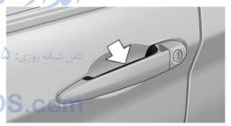
Grasp the door handle on the driver's or front passenger door completely, arrow.
