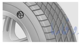
RSC label on the tire sidewall.
