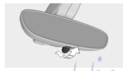
To reduce the blinding effect of the interior rear view mirror, flip the lever forward.
