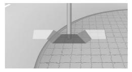
Obstacle markings can be faded into the image of the rearview camera.
