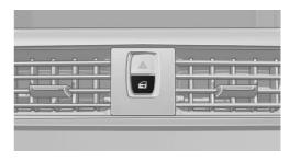
Pressing the central locking system button locks or unlocks the vehicle with the doors closed.
