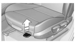
Pull the lever and move the seat to the desired tilt. After releasing the lever, apply your weight
