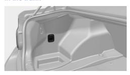
The socket is located on the left side in the trunk.
