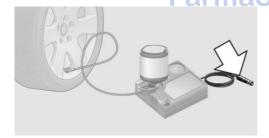
7. With the ignition turned on or the engine running, reel on the compressor.
