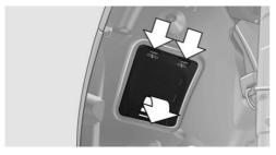
If necessary, pull the inside trim of the wheel house slightly inward. Turn the bulb socket counterclockwise and remove.
