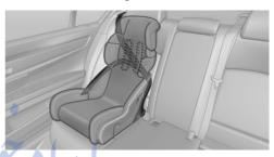
The rear safety belts and the front passenger safety belt can be permanently locked to fasten child restraint systems.
