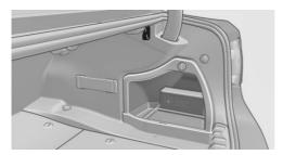
A multi-function hook is located on each side of the trunk.
