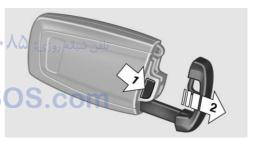
Press button, arrow 1, and remove the key, arrow 2.
