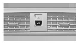
Pressing the central locking system button locks or unlocks the vehicle with the front doors closed.
