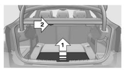
Raise the cargo floor panel, arrow 1, and latch at top, if needed, arrow 2.
