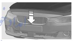
Let the hood drop from a height of approx. 16 in/40 cm and push down on it to lock it fully.
