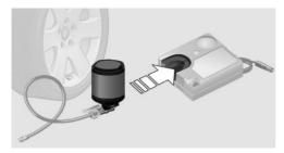
Screw the connection hose onto the tire valve of the defective wheel.
