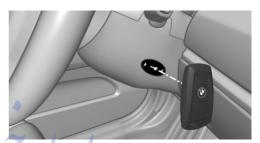
Steptronic transmission: if a corresponding Check Control message appears, hold the remote control, as shown, against the marked area on the steering column and press the Start/Stop button within 10 seconds while pressing the brake.
