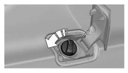
Place the tank lid in the bracket attached to the fuel filler flap.
