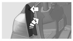
Use the screwdriver handle to loosen the two nuts, arrows 1 and 2, and remove. The tail lamp is still attached to a rubber mount on the outside.
