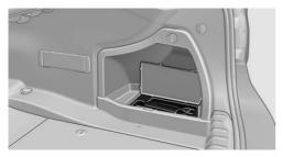
The tow fitting is in the onboard vehicle tool kit located in a storage compartment on the right side in the trunk. Open the cover.
