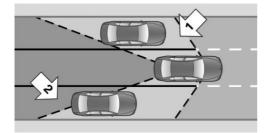
Two radar sensors below the rear bumper monitor the area behind and next to the vehicle at speeds above approx. 30 mph/50 km/h.
