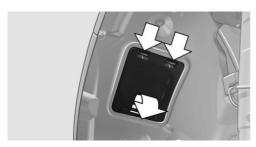
In the wheel house, loosen the two brackets and remove the cover.
