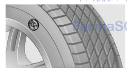
RSC label on the tire sidewall.
