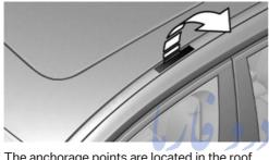
The anchorage points are located in the roof drip rail above the doors.
