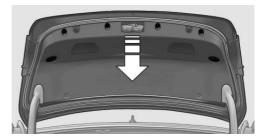
Carefully loosen the trim from the trunk lid, starting at the edge and working toward the area around the recessed grips. Make sure that the trim does not become stuck.
