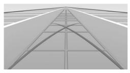
2. Turn the steering wheel to the point where the pathway line covers the corresponding turning radius line.
