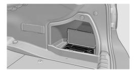
The tow fitting is in the onboard vehicle tool kit located in a storage compartment on the right side in the trunk. Open the cover.
