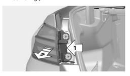
Release the catch at the top on the connector of the connecting line and remove the connector from the bulb holder.
