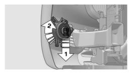
Insert the new bulb, connect the connector and screw on the wheel house panel.
