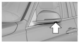
The lenses of the Top View camera are located at the bottom in the mirror housings. The image quality may be impaired by dirt.
