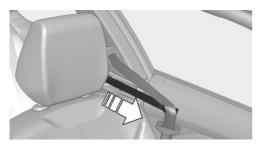
After the door is closed and the vehicle key has been detected in the car's interior, the belt carrier extends automatically and keeps the safety belt ready to put on, arrow. After the belt is put on, it goes back into the idle position.
