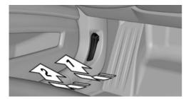
After the lever is released, pull the lever again, arrow 2.
