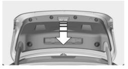
Press together hinge trim, see arrow, to release the clips.
