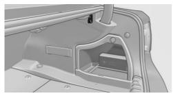
A multi-function hook is located on each side of the trunk.
