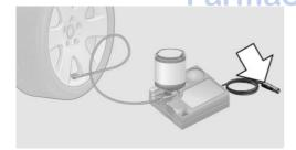
7. With the ignition turned on or the engine running, reel on the compressor.
