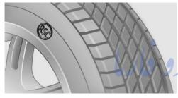
RSC label on the tire sidewall.
