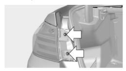
Grasp the inner edge of the tail lamp, arrow 1, and carefully pull it backward and out, arrow 2. Use your free hand to hold it in place in order to prevent the tail lamp from coming loose suddenly. Make sure
