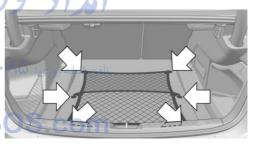
Hook the floor net into the fittings in the trunk floor.
