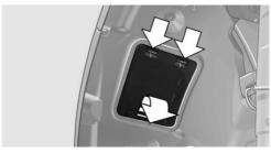
2. If necessary, pull the inside trim of the wheel house slightly inward. Turn the bulb socket counterclockwise and remove.
