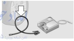
3. Attach the connection hose to the connector of the sealing container, ensuring that it engages audibly.
