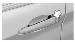
Touch the surface on the door handle of the driver's or front passenger door, arrow, with your finger for approx. 1 second without grasping the door handle.
