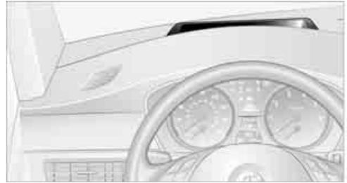
**!** Only clean the cover of the Head-Up Display with a soft, lint-free cloth or with a display cleaning cloth, as otherwise damage may result. ◀
