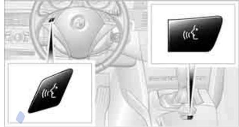
This symbol on the Control Display and an acoustic signal tell you that the voice command system can respond to commands.
