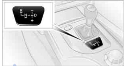
The current selector lever position is displayed on the center console.
