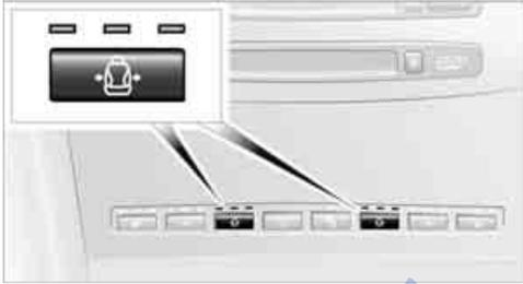
First set a comfortable backrest width, see above. Based on the backrest width set, the lateral support is automatically adapted to the current driving situation.
