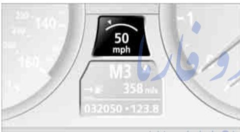
Press the lever forward **1** at a driving speed of more than approx. 20 mph/30 km/h: The system applies and stores your current speed as a desired speed. This speed is indicated on the speedometer and displayed briefly in the instrument cluster.
