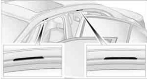
The mounting points are located in the door openings.
