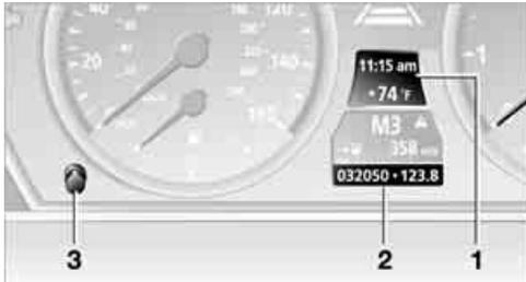
When the ignition is off you can briefly activate the time, outside temperature and odometer displays by pressing the knob **3** in the instrument cluster.
