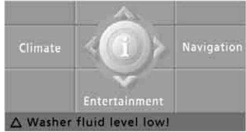
All warning lamps and indicator lamps not yet listed are also accompanied by text messages on the Control Display. These may contain more information as to the cause of a malfunction and instructions on what to do.
