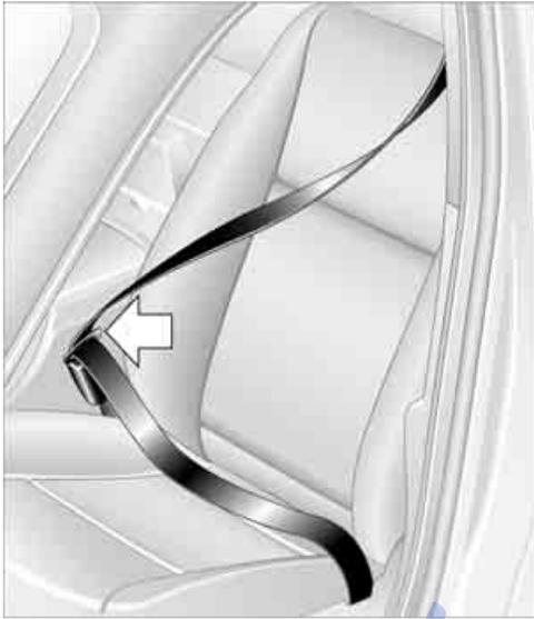
The two rear safety belt buckles integrated into the rear seat are for passengers sitting on the left and right. The belt buckle embossed with the word CENTER is intended exclusively for use by passengers riding in the center position.
