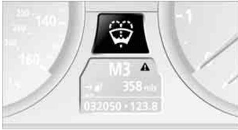
▲ This symbol means that a Check Control message has been generated. The symbol remains even if the message has been automatically masked after a short time, but is still in memory.
