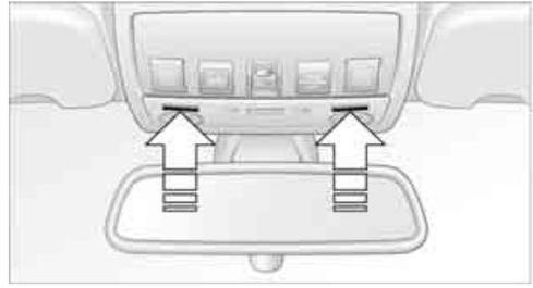
Reading lamps are provided in the front and rear adjacent to the interior lamps. Press the button to activate or deactivate this system.
