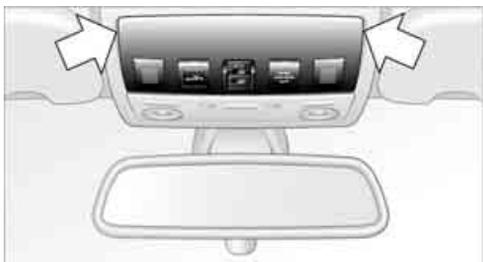
2. Insert the Allen wrench supplied with the onboard tool kit, refer to page 182, into the opening provided. Move the glass sunroof in the desired direction. The arrow below indicates the rotation direction for closing.
