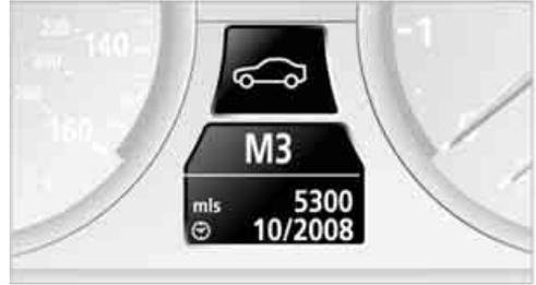
The remaining travel distance and the date for the next maintenance are displayed briefly when the ignition key is in position 2.
