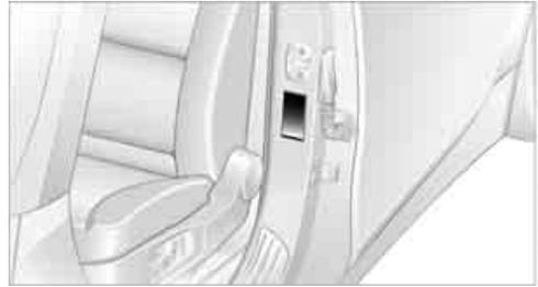
The inflation pressures for your standard tires at ambient temperature can be found on the door post when you open the driver's door.
