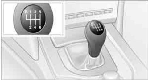
**⚠** When shifting into 5th/6th gear, press the selector lever toward the right, otherwise an inadvertent shift into 3rd or 4th gear could damage the engine. ◀
