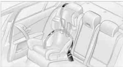
All of the rear belt retractors and the front passenger safety belt can be locked for mounting and securing child-restraint systems.
