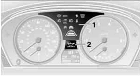
Indicator and warning lamps and their combinations are displayed in the display region 1 and in the display 2. To better differentiate between malfunctions, different symbols can be shown on the display 2.
