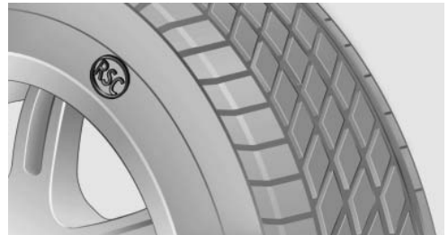
RSC label on the tire sidewall.
