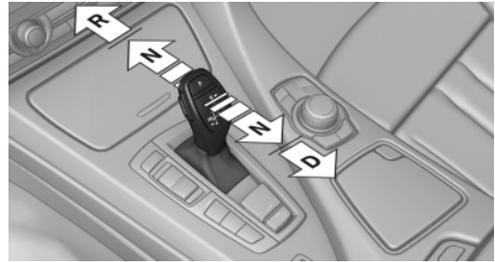
Briefly push the selector lever in the desired direction, beyond a resistance point if necessary. After releasing the selector lever, it returns to its center position.
