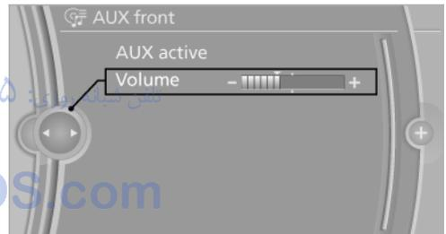
5. Turn the controller until the desired volume is set and press the controller.
