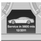
The driving distance or the time to the next service is displayed briefly after the ignition is switched on.
