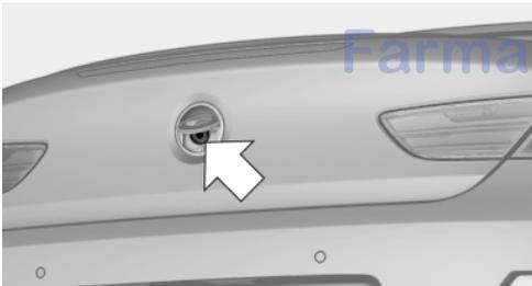
The camera lens is located under the BMW emblem of the trunk lid. The image quality may be impaired by dirt.
