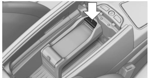
2. Insert the snap-in adapter at the front, arrow 1, and press down, arrow 2, until it engages.
