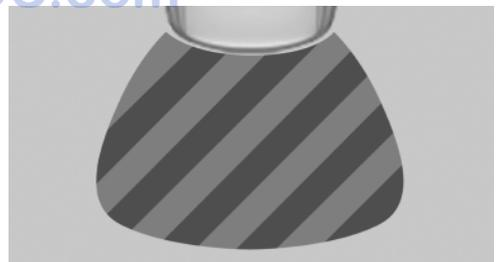
On the Control Display, the areas in front of and behind the vehicle are shaded. PDC has failed. Have the system checked.
