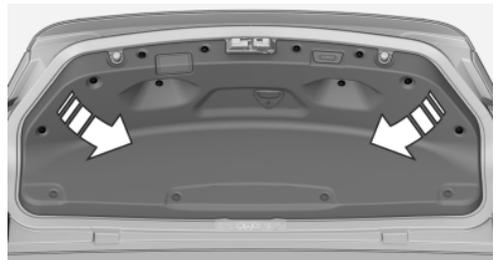
If necessary, remove the fasteners using the screwdriver from the onboard vehicle tool kit and fold away the cover.
