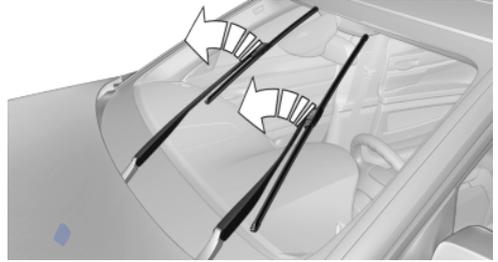
3. Position the wiper blade in a horizontal position.
