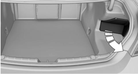
2. Pull the green knob with the fuel pump symbol. This releases the fuel filler flap.
