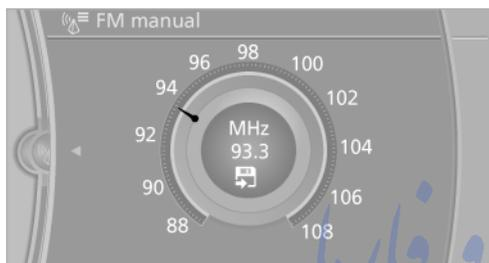
To store the station: press the controller for an extended period.
