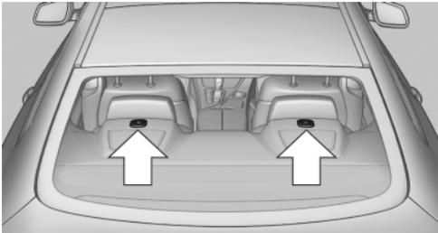
There are two mounting points for child restraint fixing systems with a tether strap.
