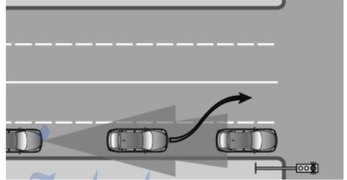
If a vehicle ahead of you unexpectedly moves into another lane from behind a stopped vehicle, you yourself must react, as the system does not react to stopped vehicles.
