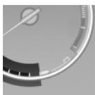
Displays the current fuel consumption. You can check whether you are currently driving in an efficient and environmentally-friendly manner.
