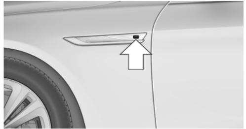
The ultrasounds sensors used to measure parking spaces are located in the side turn signals.
