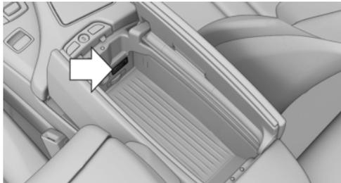
This can be used to connect an external audio device, such as an MP3 player.
