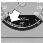
When destination guidance is activated in the navigation system, the range up to the destination is displayed.
