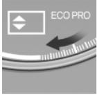
The arrow indicates that the driving style can be adjusted to be more fuel efficient by backing off the accelerator.
