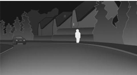
The pedestrian detection and warning system only operates in darkness and only when a heat image is displayed.
