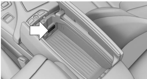
The AUX-IN port is located in the center armrest. Connect the headphones or line-out connector of the device to the jack plug.
