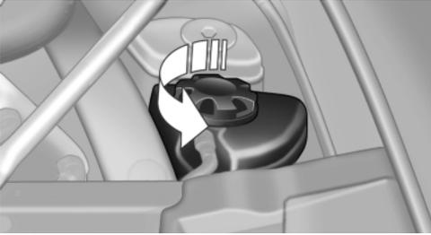
3. The coolant level is correct if it lies between the minimum and maximum marks in the filler neck.
