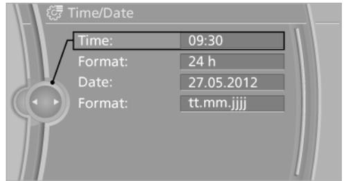
4. Turn the controller until the desired hours are displayed.
