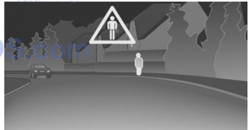
If the system detects a person in the defined area in front of the vehicle and if there is the danger of a collision with this person, a warning symbol appears in the Control Display and Head-up Display.
