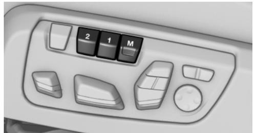
Two different driver's seat, exterior mirror, and steering wheel positions can be stored and retrieved for each remote control. The adjustment of the lumbar support is not stored.
