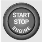
Pressing the Start/Stop button switches the ignition on or off and starts the engine.
