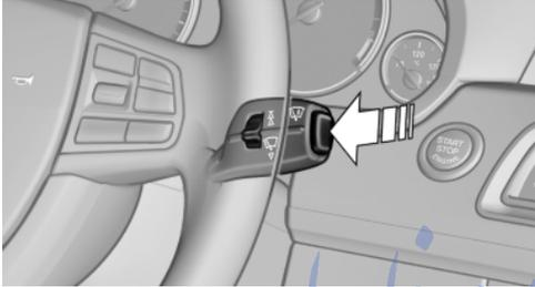
Press the button on the wiper lever.
