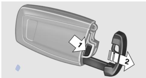
Press the button on the back of the remote control, arrow 1, and pull out the key, arrow 2.
