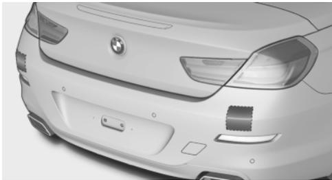
The radar sensors are located under the rear bumper.
