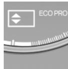
In the tachometer, a mark in the bar indicator indicates the current efficiency of the driving style corresponding to the accelerator pedal position.
