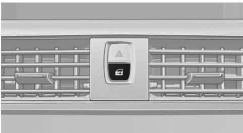
Pressing the buttons locks and unlocks the doors and the trunk lid when the doors are closed, but they are not secured against theft.
