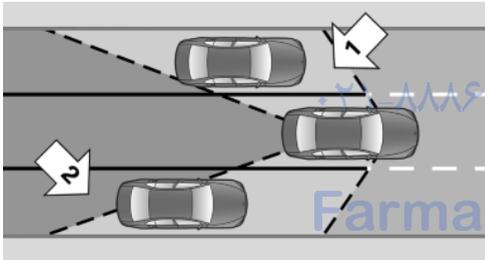
Two radar sensors below the rear bumper monitor the area behind and next to the vehicle at speeds above approx. 30 mph/50 km/h.
