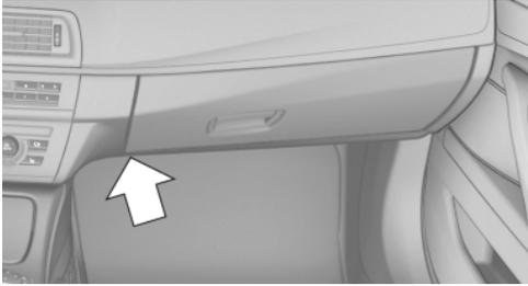
Socket is located below the glove compartment. To access the socket: fold open the cover.
