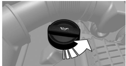
When the indicator lights up in the instrument cluster, add 1 US quart/liter of engine oil within the next 125 miles/200 km.
