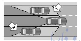
Two radar sensors below the rear bumper monitor the area behind and next to the vehicle at speeds above approx. 30 mph/50 km/h.
