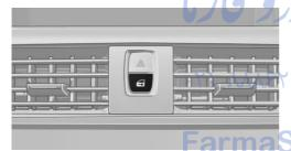
Pressing the buttons locks and unlocks the doors and the trunk lid when the doors are closed, but they are not secured against theft.
