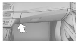
Socket is located below the glove compartment.
