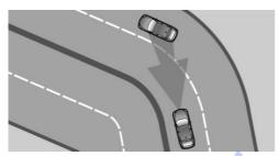
When approaching a curve, the system may react briefly to the vehicles in the next lane due to the bend of the curve. Any deceleration of the vehicle by the system can be compensated for by briefly accelerating. After the accelerator pedal is released, the system becomes active again and independently controls the speed.
