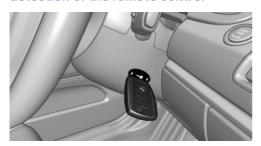
Automatic transmission: if a corresponding Check Control message appears, hold the remote control, as shown, against the marked area on the steering column and press the Start/Stop button within 10 seconds while pressing the brake.
