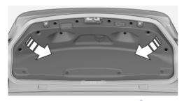
If necessary, remove the fasteners using the screwdriver from the onboard vehicle tool kit and fold away the cover.
