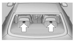
There are two mounting points for child restraint fixing systems with a tether strap.
