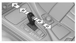
Briefly push the selector lever in the desired direction, beyond a resistance point if necessary.
