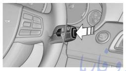
Press the button on the wiper lever.
