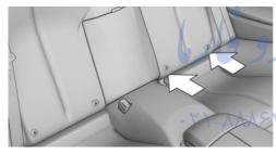
Mounts for the lower LATCH anchors are located in the gap between the seat and backrest.
