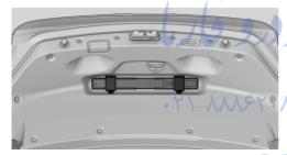
The warning triangle is located on the inside of the trunk lid.
