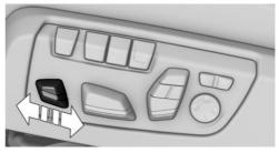
Adjust the position using the lever.
