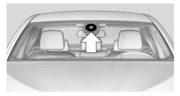
The camera is located near the base of the mirror.
