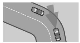
If the desired speed is too high for a curve, the speed is reduced slightly in the curve, although curves cannot be anticipated in advance.
