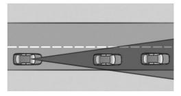
Vehicles are observed when they are traveling in the same direction of movement if they are located within the detection range of the system.
