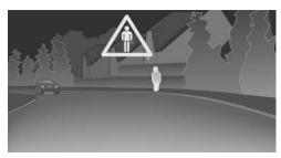
If the system detects a person in the defined area in front of the vehicle and if there is the danger of a collision with this person, a warning symbol appears in the Control Display and Head-up Display\*.
