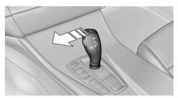
Push the selector lever to the left out of transmission position D.
