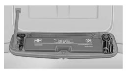
The tool kit is located in a fold-down cover in the trunk lid.
