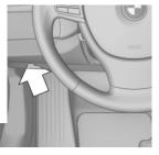
There is an OBD socket on the driver's side for checking the primary components in the vehicle emissions.
