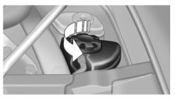
3. The coolant level is correct if it lies between the minimum and mar filler neck.
