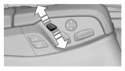
In addition, the height of the head restraint lectrically.
