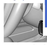
If a corresponding Check Control message appears, hold the remote control, as shown, against the marked area on the steering column and press the Start/Stop button within 10 seconds while pressing the brake.
