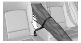
6. Tighten the retaining strap.
