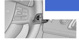
Press the button on the wiper lever.
