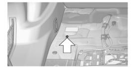
Forcefully pull the release tool up against the resistance until you notice a marked increase in the resistance and the parking brake releases audibly.  Press the switch while the brake is depressed or transmission position P is engaged.
