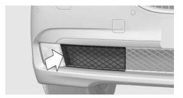
2. Remove the screw using a screw driver.
