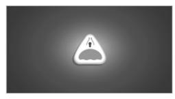
Pull the handle inside the cargo area. The trunk lid unlocks.
