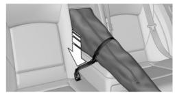
6. Tighten the retaining strap.
