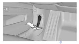
Press the release handle and open the hood.
