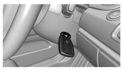
If a corresponding Check Control message appears, hold the remote control vertically against the marked area on the steering column and press the Start/Stop button within 10 seconds while pressing the brake.
