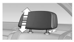
The height of the outer head restraints can be adjusted.
