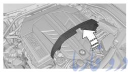
When the flap is closed, it must latch
