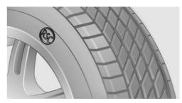
RSC label on the tire sidewall.
