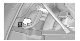
The body ground or a special nut acts as the battery negative terminal.
