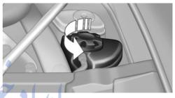
The coolant level is correct if it lies between the minimum and maximum marks in the filler neck.
