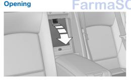
Pull on the opener and fold the cooler forward.
