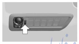
Thumbwheel for changing the air flow direction, arrow.
