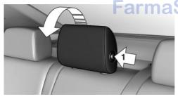
Before using the center seat, fold the center head restraint forward.
