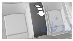
The cooler is located behind the center armrest in the rear.
