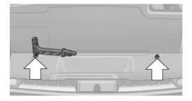
Place the release tool on the release point, arrow.
