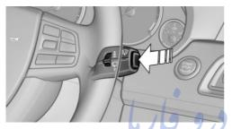
Press the button on the wiper lever.
