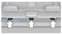
Depending on the vehicle equipment, there are two outer or three mounting points for child restraint fixing systems with a tether strap.
