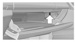
The USB interface is located in the glove compartment.
