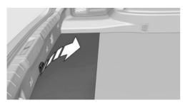
Take out the floor trim in the cargo area, removing the screws with the release tool, arrows.
