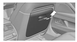
Pulling on the handle, draw the table up and out and fold it down.
