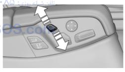
In addition, the height of the head restraint can be adjusted electrically.
