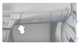
Socket is located below the glove compartment.
