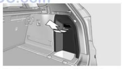
Open the cover on the right side trim and remove the sound insulation.
