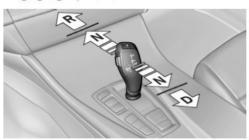
Briefly push the selector lever in the desired direction, beyond a resistance point if necessary. After releasing the selector lever, it returns to its center position.
