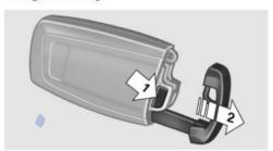
Press the button on the back of the remote control, arrow 1, and pull out the key, arrow 2.
