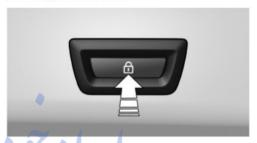
Press the button on the inside of the tailgate. When the driver's door is closed, the vehicle is completely locked.
