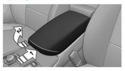
Press the button, arrow 1, and fold the center arm rest up, arrow 2.
