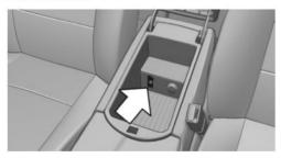
The AUX-IN port is located in the center armrest. Connect the headphones or line-out connector of the device to the jack plug.
