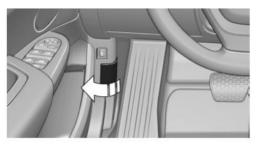
There is an OBD socket on the driver's side for checking the primary components in the vehicle emissions.
