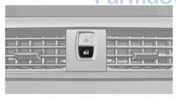
Pressing the buttons locks and unlocks the doors and the tailgate when the front doors are closed, but they are not secured against theft.
