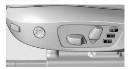
Two different driver's seat and exterior mirror positions can be stored and retrieved for each remote control. Settings for the backrest width and lumbar support are not stored in memory.
