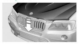
Let the hood drop from a height of approx. 16 in/40 cm and push down on it to lock it fully. Make sure you hear the engine compartment lid engage.
