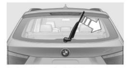
Attach a new wiper blade. It must engage audibly.
