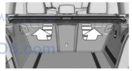
Reach under the cover and turn it upward, arrows. Pull the cover back horizontally.
