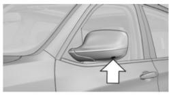
The lenses of the Top View cameras are located at the bottom of the exterior mirror housings. The image quality may be impaired by dirt. Clean the lens, refer to page 268.
