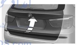
Press the button on the exterior of the tailgate.
