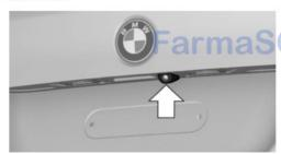
The camera lens is located in the handle of the tailgate. The image quality may be impaired by dirt.
