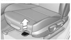
Pull the lever and move the seat to the desired tilt. After releasing the lever, apply your weight to the seat or lift it off to make sure the seat engages properly.
