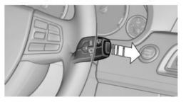
Press the lever forward: intermittent wipe. When reverse gear is engaged, the system switches to continuous operation.
