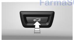
Press the button on the inside of the tailgate. The tailgate closes automatically. Pressing again stops the motion.
