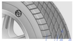
RSC label on the tire sidewall.
