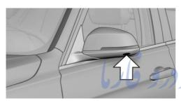
The lenses of the Top View cameras are located at the bottom of the exterior mirror housings. The image quality may be impaired by dirt.
