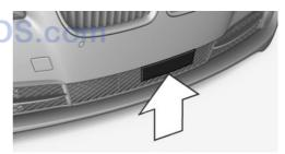
The radar sensor is located in the lower area of the front bumper.
