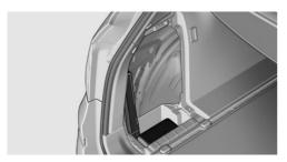
The tow fitting is located in the onboard vehicle tool kit behind the left folding cover in the trunk.
