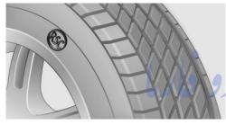
RSC label on the tire sidewall.
