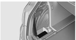
The warning triangle is located behind the lefthand cover in the trunk.
