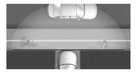
Side View provides an early look at cross traffic at blind driveways and intersections. Road users concealed by obstacles to the left and right of the vehicle can only be detected relatively late from the driver's seat. To improve the viewing, each camera, front and rear on the vehicle, detects the traffic area on the side.
