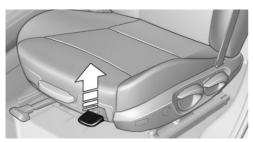
Pull the lever and move the seat to the desired tilt. After releasing the lever, apply your weight
