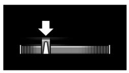
The mark in the efficiency display is backlit in blue and is located at the zero point. The tachometer approximately indicates idle speed.
