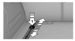
To slide the lashing eyes, press the button, arrow 1. Make sure that the lashing eyes latch at the new position.
