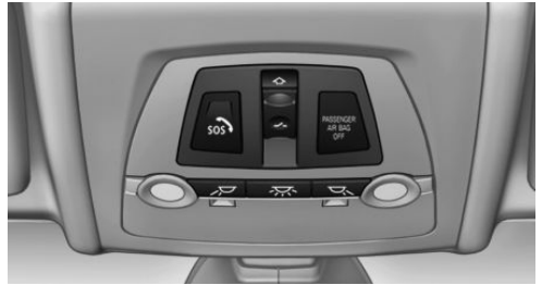
SOS button in the roofliner
