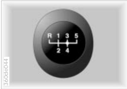
Press the clutch pedal all the way down each time you shift, pressing the gear-shift lever into its proper end position.
