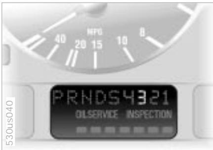
You can drive as with a normal automatic transmission. In addition, you can also shift manually.
