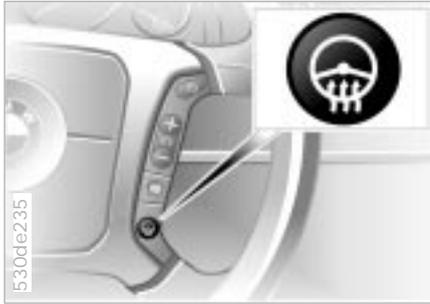
Steering wheel heating functions in ignition key position 2.
