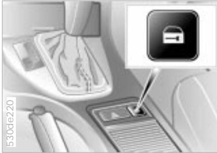
You can operate the central locking system with this button when the driver's door is closed. The doors and liftgate are unlocked or locked only. However, the anti-theft system is not activated. Also, the fuel filler door remains unlocked to allow refueling.
