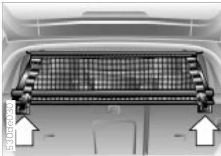
6. Attach the hooks on the bottom of the partition net into the eyes on both sides
