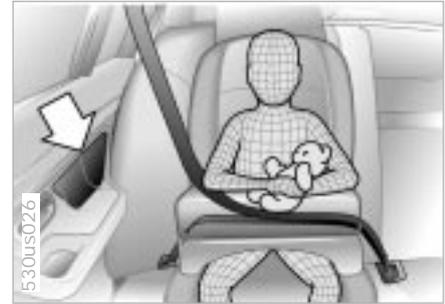
This is the right way a child should sit in a child-restraint device when rear side airbags (arrow) are provided.
