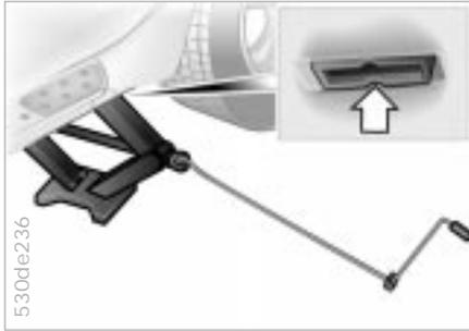
5. Position the jack at the jacking point closest to the flat tire so that the jack base is vertically below the jacking point and the entire surface of the head of the jack will move into the square recess of the jacking point (refer to the illustration detail) when the jack is cranked
