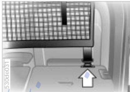
7. When the rear backrests are folded down, you can open the Velcro® strips, completely unroll the partition net, insert it in the front retainers on the roof and attach the three hooks into the eyes.
