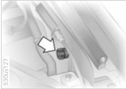
6. Next, connect one end of the other jumper cable (-) to either the support vehicle's negative battery terminal or a suitable ground on its engine or bodywork. Connect the other end to the negative battery terminal or a suitable ground on the vehicle being started. There is a special nut for this on the left side panel of your BMW. Refer to the arrow in the illustration
