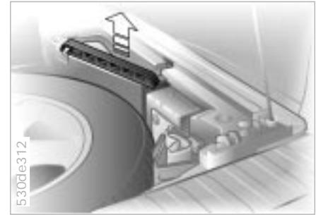
4. Remove the support rod from the bracket
