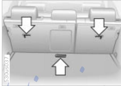
If you use a child-restraint system with a tether strap, three additional tether anchorage points (refer to the arrows in the illustration) have been provided. Depending on the location selected for seating in the rear passenger area, attach the tether strap to the corresponding anchorage point to secure the child-restraint system. Remove the cover first on the middle location.
