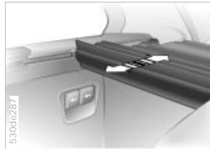
When the cover is pulled out, it can be opened behind the rear-seat backrest to gain access to the cargo area from the rear seats during a trip, for example.
