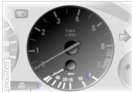
Indicates the current fuel consumption in mpg (in liters/100 km on Canadian vehicles). This allows you to see whether your current driving style is conducive to fuel economy with minimum exhaust emissions. *تلفن شبانه رو*
