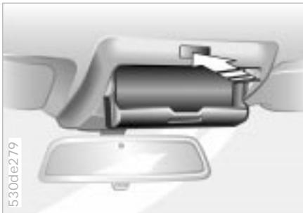
Press the button to open; fold upward to close.
