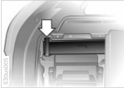
1. Open the cover on the left in the cargo area: lift the handle on the cover
