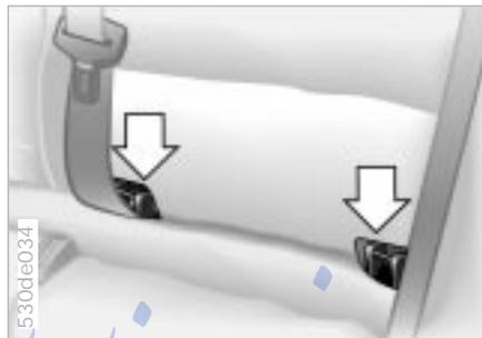
The illustration shows the mounts for a LATCH child-restraint system in the left rear seat.
