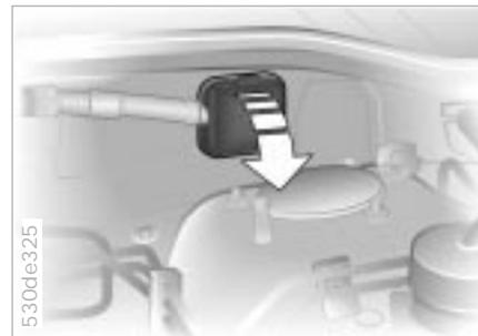
5. Use one jumper cable (+) to connect the positive terminal of the battery in the support vehicle with the auxiliary positive terminal provided in the engine compartment of your BMW specifically for jump starting. The cover on this auxiliary terminal is identified by a "+" symbol, refer to the illustration. To remove the cover, tip up the cap (arrow)
