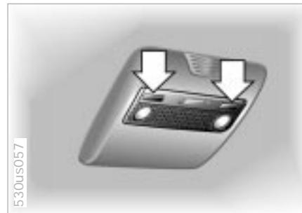
Reading lamps are provided in the front and rear\* near the interior lamp. They can be switched on and off with the button (arrows) next to each lamp.
