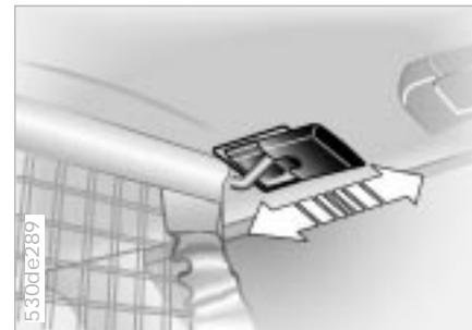
3. Slide back the covers on the retainers for the partition net on both sides of the roof (arrow)
