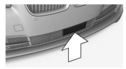
Always keep radar sensor clean and unobstructed.
