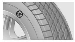
RSC label on the tire sidewall.
