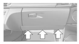
Loosen fasteners, arrows, and open cover.
