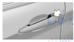
Touch the surface on the handle of a vehicle door, arrow, with your finger and hold it there without grasping the door handle.
