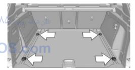
To secure the cargo there are four movable lashing eyes in the cargo area.
