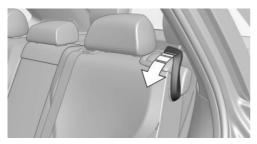
2. Pull the lever and fold the seat forward. If the second row of seats is not locked, a warning symbol is displayed in the instrument cluster.
