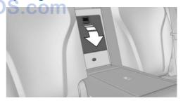
Pull on the opener and fold the cooler forward.
