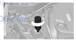
Press the bottle down, see arrow. The vehicle tank will be filled. The tank is full when the fill level in the bottle no longer changes. It is not possible to overfill.
