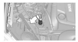
The fuel cap for the Diesel exhaust fluid is located in the engine compartment.
