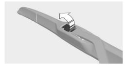
Slide wiper blade out of the wiper arm.
