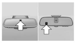
Photocells are used for control:
