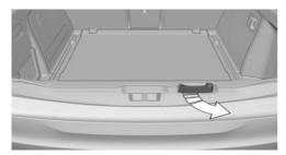
Pull the lever and swing down the tailgate. The open tailgate can be loaded with up to 550 lbs/250 kg.
