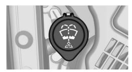
All washer nozzles are supplied from one reservoir in the engine compartment.
