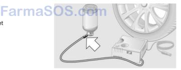
4. Insert the sealant container on the compressor housing in an upright position.
