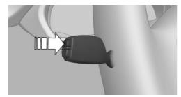
Press and hold PC button on blinker lever.
