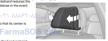
Fold forward for increased lateral support in the resting position.
