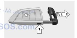
Press button, arrow 1, and remove the key, arrow 2.
