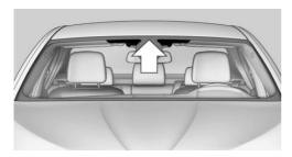
The marked area is not covered with heat reflective coating. Use this area for garage door openers, devices for electronic toll collection, etc.
