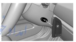
If a respective Check Control message appears, hold the remote control with its back against the marked area on the steering column. The tailgate button on the remote control should be at the same height as the marked area. Press the Start/Stop button within 10 seconds while pressing the brake pedal.
