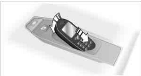
The mobile phone battery is charged from the radio readiness position.
