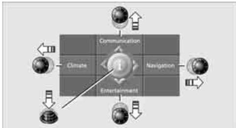
With the start menu you can open the menu items Communication, Navigation, Entertainment and Climate by moving the controller to the left, right, front or rear.
