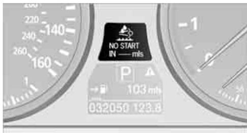
Even with a display of -- mls, the engine will continue to run, provided that it is not switched off, and all other operating requirements are met, e.g. sufficient fuel.
