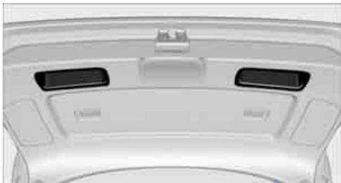
The handle recesses on the interior trim of the liftgate make it easier to pull down.
