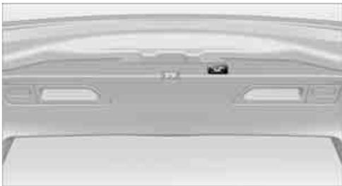
The liftgate closes automatically when you press the button on the inside of the liftgate.
