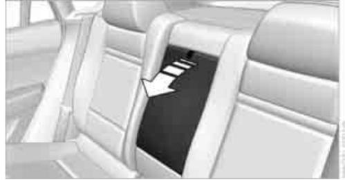
Pull on the loop and fold down the center armrest.
