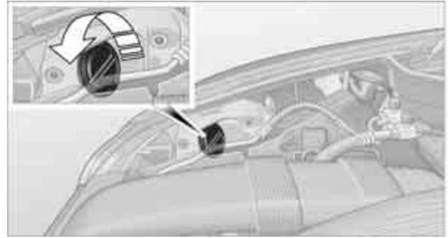
2. Turn the bulbs to the left, pull off the connector and replace.
