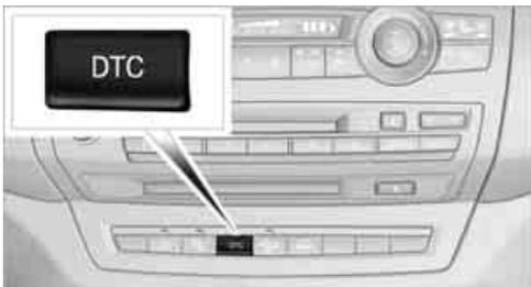
Press the button briefly; the DTC indicator lamp in the instrument panel lights up.
