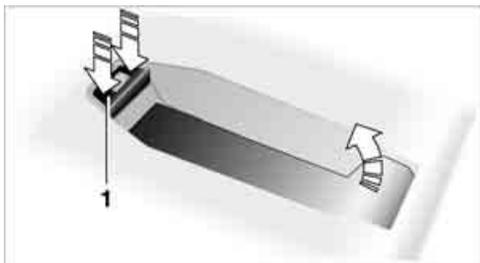
2. Insert the snap-in adapter in the front and press it downward until it engages.
