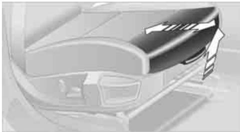
Pull the lever and adjust the thigh support in the longitudinal direction.
