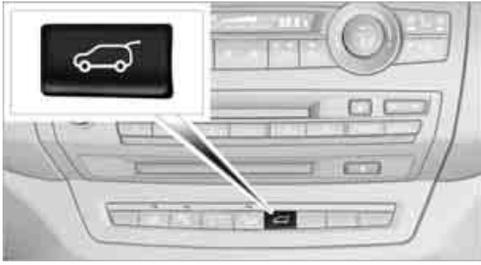
Press the button: the liftgate opens somewhat unless it has been locked.
