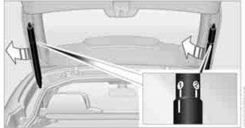
For the upper position, position 2: Turn sleeves of both liftgate supports in the direction of the arrow until the line markings align in position 2.
