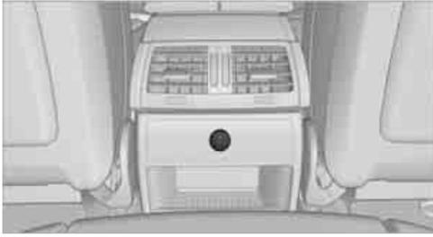
Depending on your vehicle's equipment package, the socket in the rear is covered with a cap or equipped with a lighter. Refer to Cigarette lighter, front, page 129.
