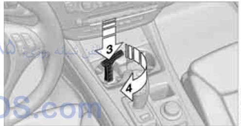
5. Turn the releasing tool as far as possible, arrow 4, and then press downward and leave it in. The transmission lock is released.
