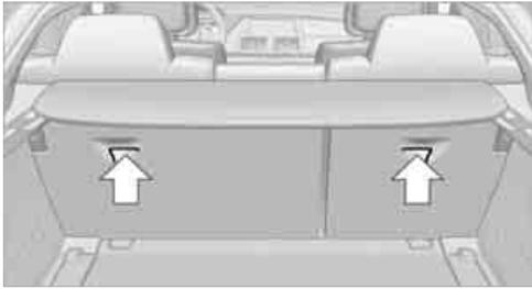
For child restraint devices with tether strap, there are two additional attachment points on the back of the rear seat backrests, refer to arrows.
