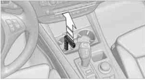
1. Pull out the releasing tool. The transmission lock is engaged again.
