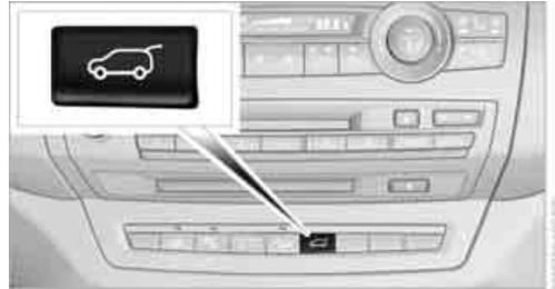
Press the button: the liftgate opens somewhat unless it has been locked.
