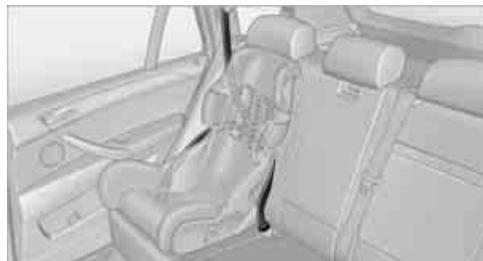
The rear safety belts, in the BMW X5 all of the safety belts of the 2nd and 3rd\* row seats and the passenger safety belt can be locked to prevent them from being pulled out in order to secure child restraint devices.
