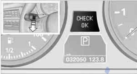
1. Press the button on the turn signal lever downward. "CHECK OK" or the stored Check Control messages appear in the display. "CHECK OK" is shown if no messages are present. Check Control messages are accompanied by text messages on the Control Display.
