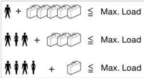
The permissible load is the total of the weight of occupants and cargo/luggage. The greater the weight of occupants, the less cargo/luggage can be transported.
