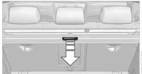
Pull out the roll-up cover and hook it into the brackets.
