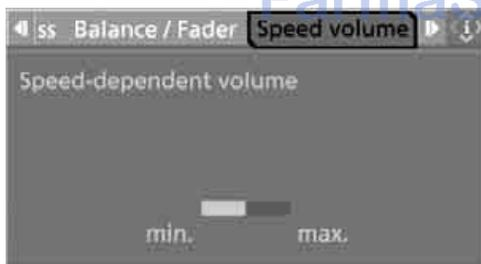
2. Turn the controller: The adjustment is applied; the field can be changed.
