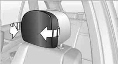
You can fold the side extensions on the head restraint forward for increased lateral support in the resting position.
