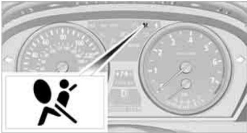
From radio readiness, refer to page 65, the warning lamp lights up briefly, indicating the operational readiness of the entire airbag system and the safety belt tensioners.
