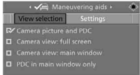
7. Select "PDC in main window only" and press the controller.
