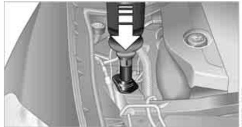
3. The reservoir is full when the fill level in the bottle stops changing. It is not possible to overfill.
