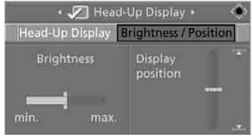
7. If necessary, move the controller to the left or right to select "Brightness" or "Display position".
