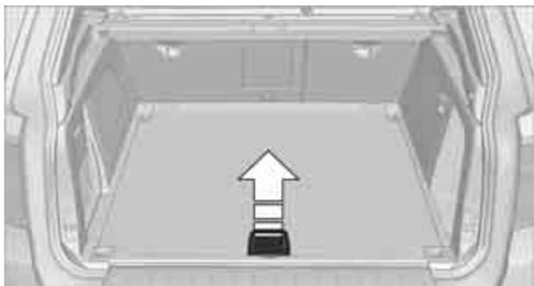
The onboard toolkit is located in the cargo bay under the floor panel.
