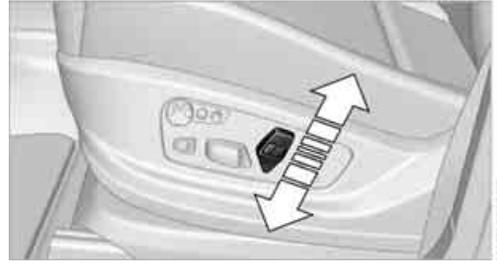
You can adjust the height of the head restraints electrically. ◀
