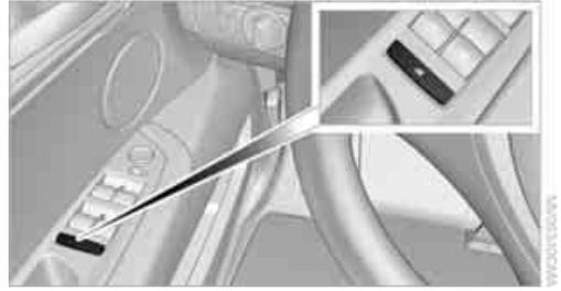
With the safety switch, you can prevent the rear windows from being opened or closed via the switches in the rear passenger area, by children, for example. The LED lights up when this safety feature is activated.
