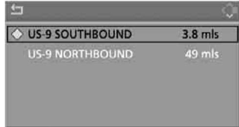
First the traffic information along the planned route is shown sorted according to the distance to the current vehicle position.
