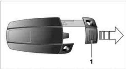
Press button 1 to unlock the key.
