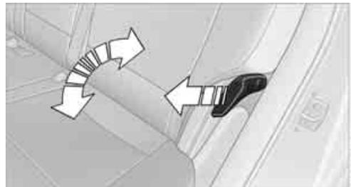
Pull the lever and apply weight to or remove weight from the backrest as needed.
