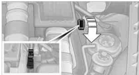
2. Attach one end of the jumper cable plus/+ to the positive terminal of the battery or a starting-aid terminal of the vehicle providing assistance.
