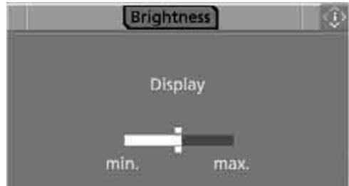
6. If necessary, move the controller to the right to select "Display".
