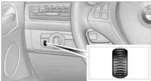
You can control the lighting intensity by using the serrated dial.
