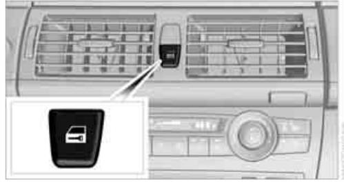
This button serves to unlock or lock doors and the liftgate, with the front doors closed. It does not activate the anti-theft system. The fuel filler door remains unlocked.
