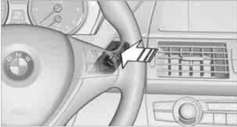
Insert the remote control as far as possible into the ignition lock. Radio readiness switches on. Some electronic systems/consumers are ready for operation.
