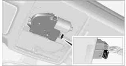
4. Insert the Allen wrench\* from the onboard tool kit, refer to page 269, into the opening provided. Move the panorama glass sunroof in the desired direction.
