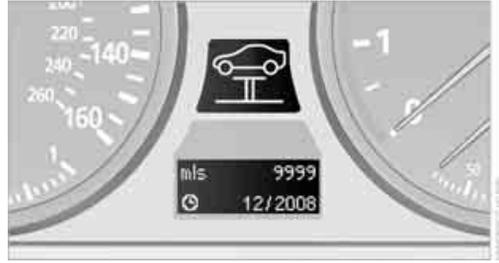
The remaining driving distance and the date for the next maintenance are displayed briefly with the ignition switched on.
