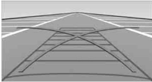
2. Turn the steering wheel so that the pathway lines cover the corresponding turning lines.
