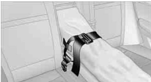
BMW X6: attach the hook of the ski bag retaining strap to the eyelet on the rear seat backrest.
