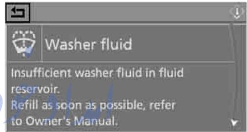
You can display additional information on most Check Control messages later, e.g. on the cause of the malfunction and on corresponding need for action, see below.
