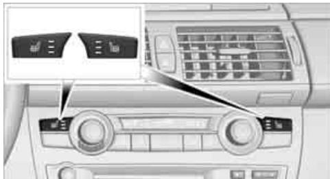
The temperature setting progresses one step through its control sequence each time you press the button. The maximum temperature is supplied when three LEDs are lit.
