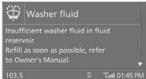
Additional information, e.g. on the cause of a malfunction and on the corresponding need to take action can be displayed via the Check Control, refer to page 85.
