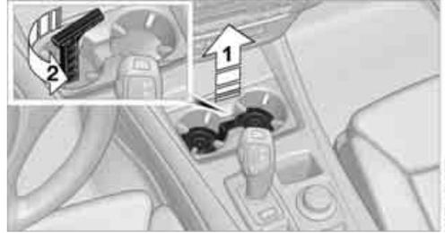
2. Open the cover in the bottom of the cup holder with the releasing tool from the onboard tool kit, page 269, refer to arrow 2.
