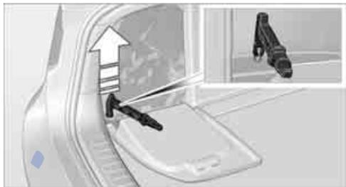
4. Firmly pull the releasing tool upward against the mechanical resistance, refer to arrow, until a considerable increase in force is felt and the parking brake is then clearly heard to release.
