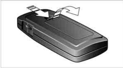
1. Press the detent and remove the cover.
