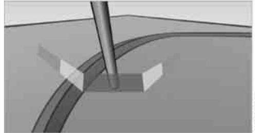
The obstacle marking is deactivated when driving in reverse from approx. 12 mph/20 km/h.
