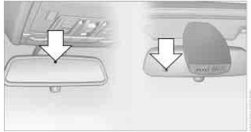
This feature is controlled by two photocells in the inside rearview mirror, one on the front and one on the back.
