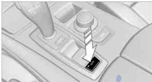
Press the button. The LED in the button lights up and the indication AUTO H appears in the instrument panel.
