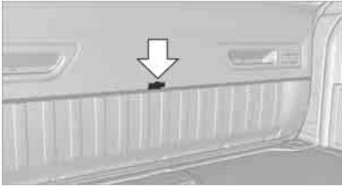
2. Open the liftgate and press in the handle. The liftgate is locked again as soon as it is closed.
