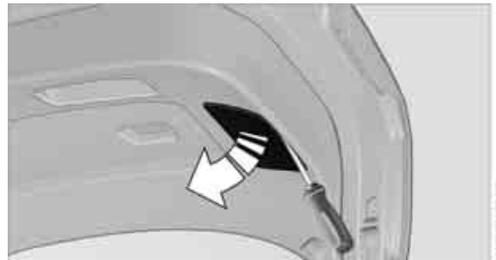
2. Rotate the bulb socket to the left and remove.
