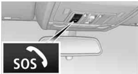
2. Press the button for at least 2 seconds. The BMW Assist Response Center is contacted.
