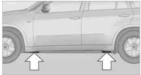
2. Guide the jack head into the rectangular recess of the jacking point when cranking up, refer to illustration detail.
