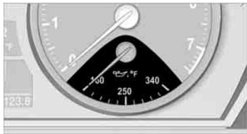
When the engine is at operating temperature, the engine oil temperature is between approx. 170 °F/80 °C and approx. 250 °F/120 °C.
