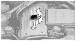
Depending on the engine, the filler neck is located in the middle, as shown, or at the front corner in the engine cover.
