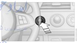
Pressing the Start/Stop button switches the radio ready state or the ignition on and off.
