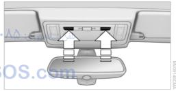
The reading lamps are located next to the interior lamp. To switch on and off, press the button.
