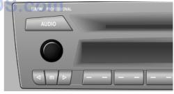
Press the left knob. The radio selects the audio source set last: radio, CD, external audio device, or USB audio interface.
