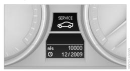
The remaining driving distance and the date of the next maintenance are displayed briefly after the ignition is switched on.
