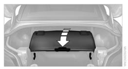
Before opening the hardtop, close the cargo area partition, arrow, and make sure it engages on both sides.
