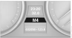
The gear position and the engaged gear, such as M4, are displayed.
