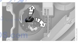
Disconnect the plug, change the bulb and reconnect the plug.
