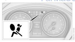
When the ignition, refer to page 46, is switched on, the warning lamp comes on briefly to indicate that the entire airbag system and the belt tensioners are operational.
