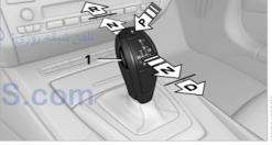
Briefly push the selector lever in the desired direction, beyond a resistance point if necessary. When shifting out of P or into R, simultaneously push the unlock button 1.
