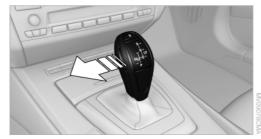
Press the selector lever from gear position D to the left to activate the Sport program.
