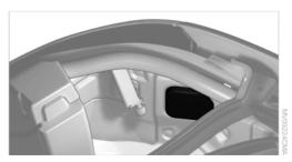
Pull out the bulb holder, see arrow, and change the bulb.
