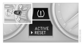
Press button 2 for approx. 5 seconds until the small warning lamp lights up yellow and the following display appears:
