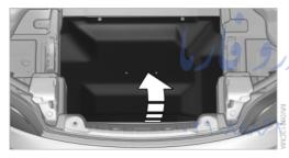
The onboard vehicle tool kit is stored in a pouch under the trunk floor panel.
