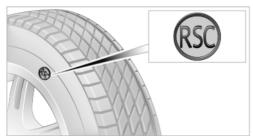
RSC label on the tire sidewall.
