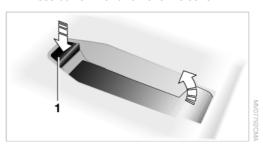
Insert the snap-in adapter at the front, arrow 1, and press down, arrow 2, until it engages.
