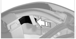
Press the locking mechanism in the trunk, see arrow, and remove the cover.
