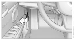
An OBD socket for testing components that are critical to exhaust composition is located under a cover on the driver's side.
