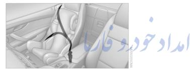
The safety belt for the passenger can be locked to prevent it from being pulled out when it is used to secure child restraint systems.
