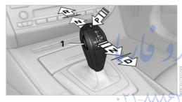
Briefly push the selector lever in the desired direction, beyond a resistance point if necessary. When shifting out of P or into R, press button 1 at the same time.
