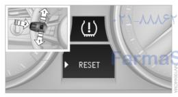
Press button 2 to confirm your choice of the Flat Tire Monitor. 4. Press button 2 for approx. 5 seconds until the display appears:
