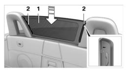
Push the wind deflector down, arrow 1, and then push down and forward simultaneously, arrow 2, until it engages.
