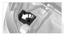
To open: turn the lock to the left, see arrow, and fold the cover up.
