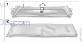
Fold the wind deflector 1 and slide it into the storage pouch 2.
