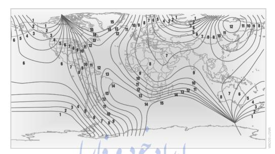
In order to set the compass zones, press and hold the adjustment button for 3-4 seconds. The number of the compass zone set is shown in the display.
