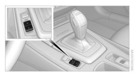
Sporty driving with optimized chassis and suspension during limited driving stabilization.
