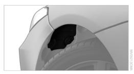
Turn both locks in the wheel house to the left and remove the cover.
