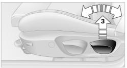
Pull lever 3 and move the backrest to the desired tilt.
