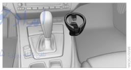
Mount the cupholder onto the center console so that it snaps into place.
