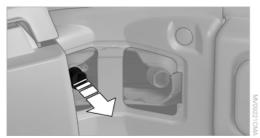
Pull out the bulb holder and replace the bulb.
