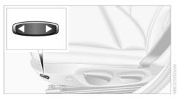
Press the front/rear section of the switch. The backrest width decreases/increases.
