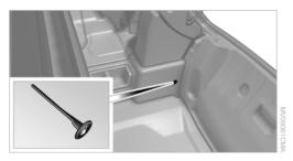
Pull the button in the trunk with the fuel pump symbol down. This releases the fuel filler flap.
