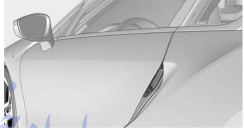
The driver's door can be opened at the door lock using the integrated key, refer to page 36.
