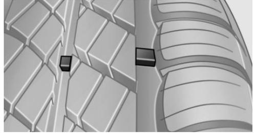
Wear indicators are distributed around the tire's circumference and have the legally required minimum height of 0.063 in/1.6 mm.
