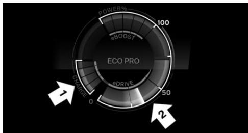
The driving style is efficient as long as the accelerator pedal pointer is within the lower range highlighted in blue during acceleration and deceleration.
