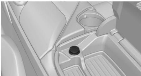
The socket is located between the front seats. Remove the cover.
