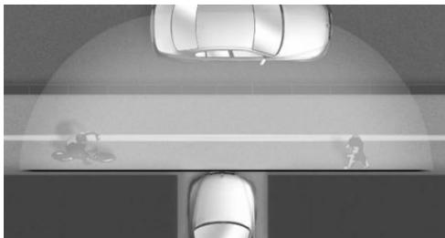
Side View provides an early look at cross traffic at blind driveways and intersections. Road users concealed by obstacles to the left and right of the vehicle can only be detected relatively late from the driver's seat. To improve the viewing, each camera, front and rear on the vehicle, detects the traffic area on the side.
