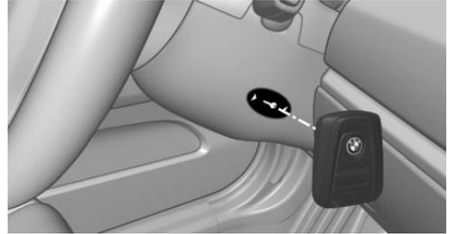
If a respective Check Control message appears, hold the remote control with its back against the marked area on the steering column. The BMW logo on the remote control should be at the same height as the marked area. Press the Start/Stop button within 10 seconds while pressing the brake pedal.
