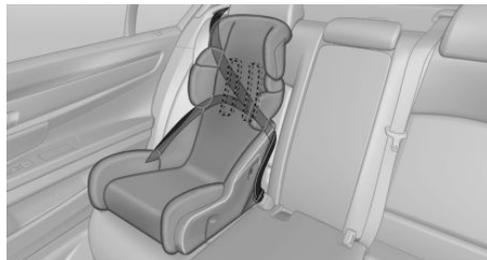
The rear safety belts and the front passenger safety belt can be permanently locked to fasten child restraint systems.
