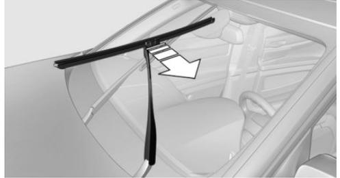
5. Insert the new wiper blade in reverse order of removal until it locks in place.
