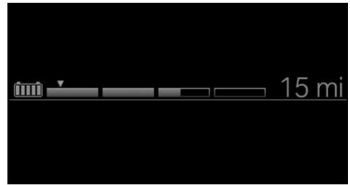
▽ In the Maintaining charging state mode, the arrow indicates the charging state of the high-voltage battery that should be conserved for a later point in the trip.
