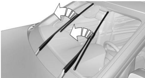
3. Position the wiper blade in a horizontal position.
