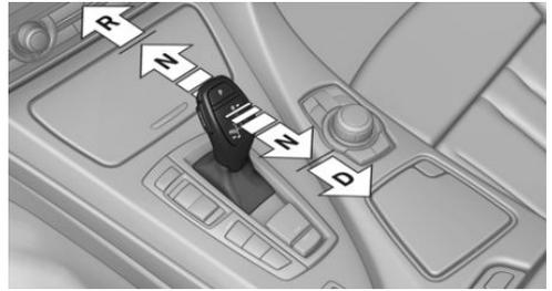
Briefly push the selector lever in the desired direction, beyond a resistance point if needed.
