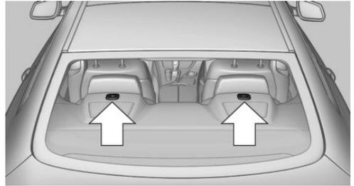
There are two mounting points, located above the respective seats, for child restraint systems with a tether strap.
