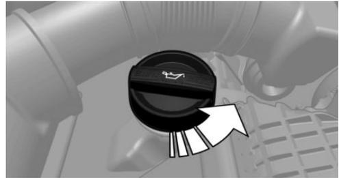
Only replenish the maximum engine oil amount of 1 US quart/liter if the signal is displayed in the instrument cluster.
