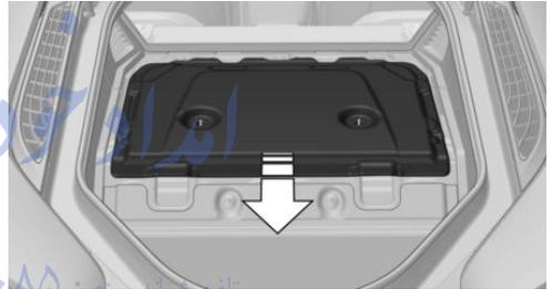
3. Turn screws counterclockwise to undo them and remove engine compartment cover, arrow .
