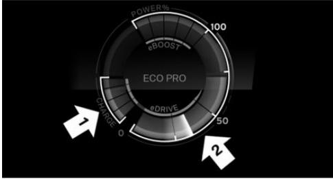
A bar display in the instrument cluster indicates your current driving efficiency.
