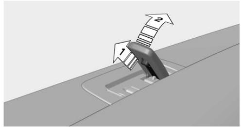
Pull the release on the bottom of the lever upwards, arrow 1, then push the lever forwards, arrow 2.
