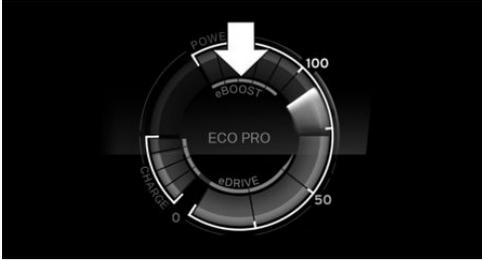
Five bars indicate the available output of the electric motor for the eBOOST acceleration boost. Depending on the available output of the high-voltage battery, there could be more or less eBOOST available. If the high-voltage battery is completely discharged, all five bars are grayed-out.
